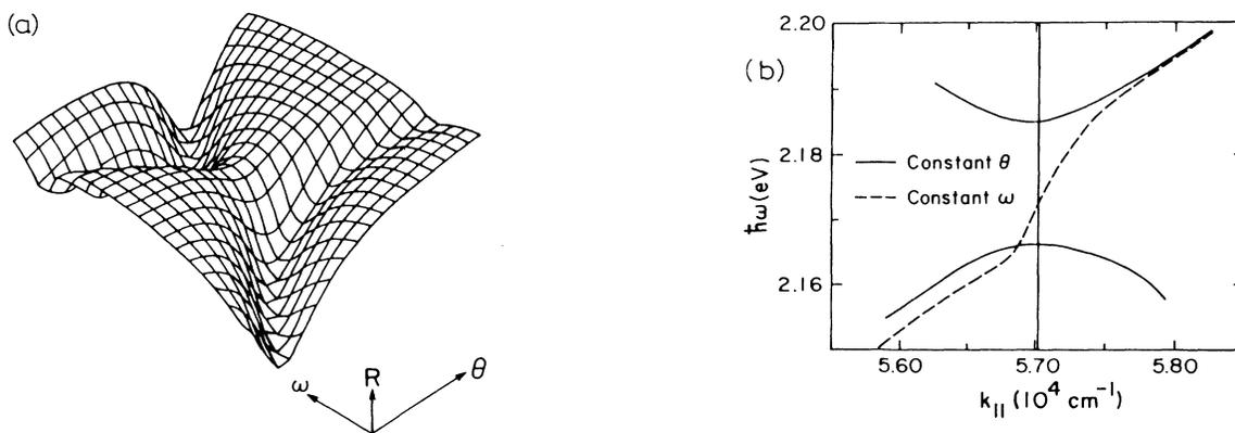
FIG. 2. (a) The reflectivity surface  $R(\omega, \theta)$  as calculated in Ref. 6 for silver on a sawtooth grating with a period  $a = 1.1 \mu\text{m}$  and amplitude  $h = 30 \text{ nm}$ . A gap is found in energy. (b) Dispersion curves deduced from the reflectivity distribution of (a) with  $\theta = \text{const}$  scans (solid line) and  $\omega = \text{const}$  scans (dashed line). No gaps are found in the latter case. (From Ref. 6.)
