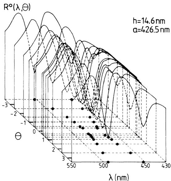
FIG. 9. Reflection of monochromatic light from a sinusoidally modulated Ag surface with periodicity  $a=426.5$  nm and modulation amplitude  $h=14.6$  nm. The spectra are measured at a fixed angle of incidence  $\theta$  in a sweep of the wavelength  $\lambda$ . The spectra have not been corrected for the smooth-spectral sensitivity of the experimental setup. The position of the reflection minima is projected onto the  $(\theta, \lambda)$  plane.
