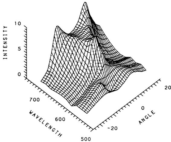
FIG. 6. Distribution of light intensity in the  $(\lambda, \theta)$  plane emitted by a silver-coated MOM diode, sinusoidally modulated with  $a=549$ -nm periodicity and with  $h=31$ -nm amplitude. Measurements were made with  $\lambda=\text{const}$  scans at  $U=+3.2$  V and  $T=-112^\circ\text{C}$ . No gaps can be seen. (For units, see Fig. 4.)
