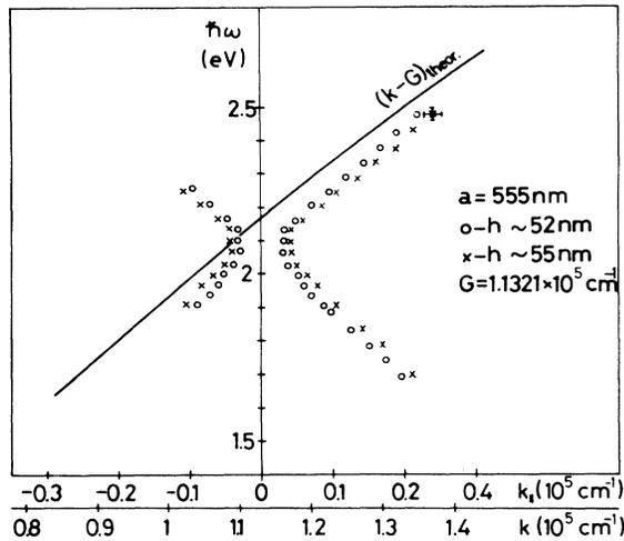
FIG. 3. Dispersion relation of SP for silver topped MOM diodes with period  $a = 555$  nm and with different amplitudes  $h$ . Tunnel emission intensity was measured in  $\omega = \text{const}$  scans at  $U = +2.5$ -V bias and at room temperature (Ref. 8).
