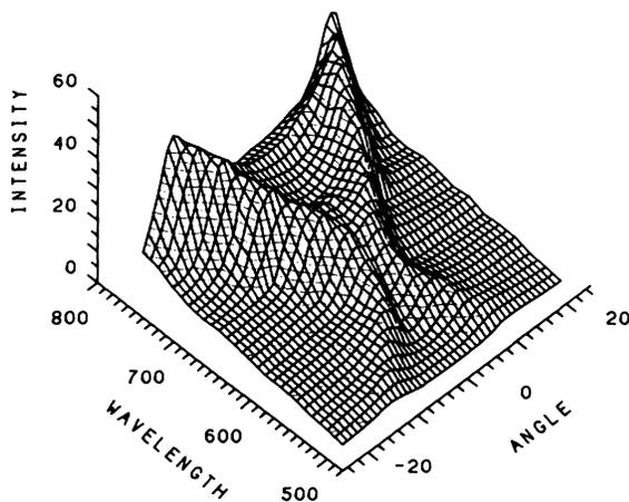
FIG. 4. Distribution of light intensity in the  $(\lambda, \theta)$  plane emitted by a silver-coated tunnel diode, modulated with  $a = 555$ -nm periodicity and with  $h = 52$ -nm amplitude. (The grating was the same as in Fig. 3.) Measurements were made with  $\lambda = \text{const}$  scans at  $U = +2.5$  V and at  $T = -106^\circ\text{C}$ . A well-defined momentum gap is observed. (Wavelength in nanometers, angle in degrees, intensity in arbitrary units.)
