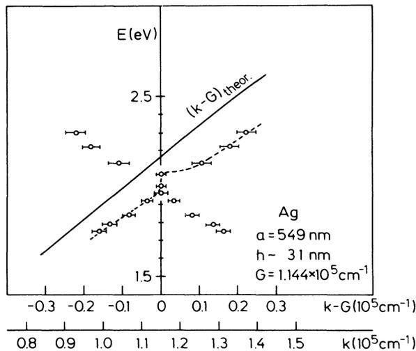
FIG. 7. SP dispersion relation determined from scans shown in Fig. 6.
