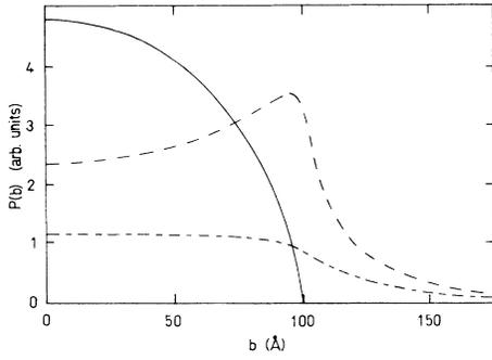
FIG. 1. Energy-loss probability as a function of impact parameter  $b$  for a 50-keV electron incident upon an aluminum sphere of radius 100 Å. Solid line: bulk mode; dashed line: total contribution of the first 20 surface modes ( $\times 6$ ); dashed-dotted line: dipole ( $l=1$ ) surface mode ( $\times 6$ ).
