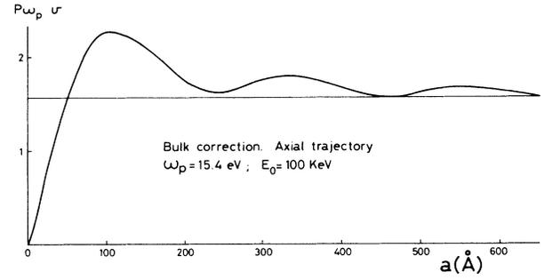
FIG. 2. Bulk correction to the plasmon excitation probability, as a function of the sphere radius for a 100 keV electron incident axially on an aluminum sphere. A free-electron  $\epsilon(\omega)$  response function has been used in the calculation.
