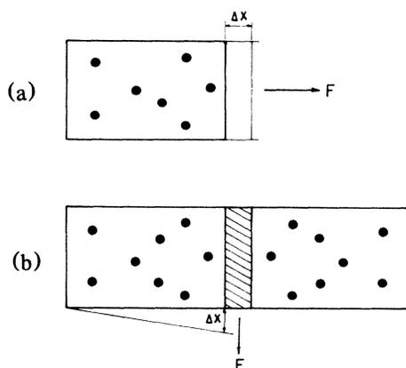
FIG. 1. Configurations of the sample in the elasticity measurements. In *b* two identical samples are used, with the holes at the same positions.  $\Delta x$  is displacement of the plate and  $F$  is the applied force.
