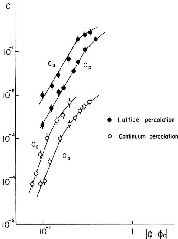
FIG. 3. Elastic constants vs  $(\phi_c - \phi)$ .  $a$  corresponds to Fig. 1(a) and  $b$  corresponds to Fig. 1(b).
