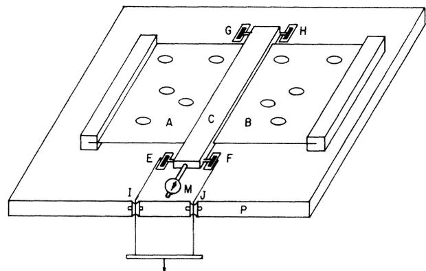
FIG. 2. Schematic view of the device for measuring the elastic constant in the configuration of Fig. 1(b). A, B are samples. P is the basis plate. C is the mobile beam. M is the micrometer. E, F, G, H, I, and J are the locations of ball bearings.
