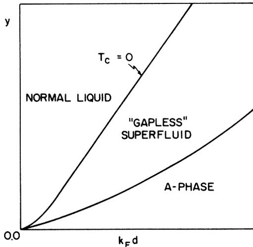
FIG. 3. The  $T=0$  phase diagram of superfluid  $^3\text{He}$  film. Quantitatively, boundaries between different regions will depend on the particular model for surface scattering but the qualitative features are expected to persist. By controlling the thickness, or by a careful choice of the substrate material, it should be possible to experimentally "open" the "window" with a view on properties of a dirty anisotropic superfluid.
