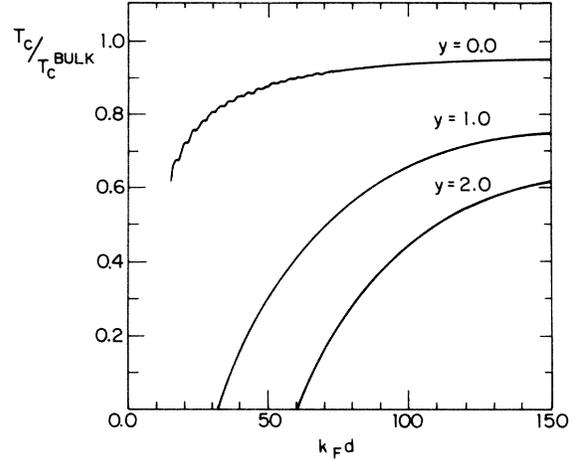
FIG. 1. Transition temperature of a superfluid  $^3\text{He}$  film as a function of thickness. Surface roughness parameter  $y$  is defined in (3.4). In an ideal ( $y=0.0$ ) film case, the wiggles in  $T_c$  are due to quantum size effects. We show results in the region  $k_F d > 15$ .
