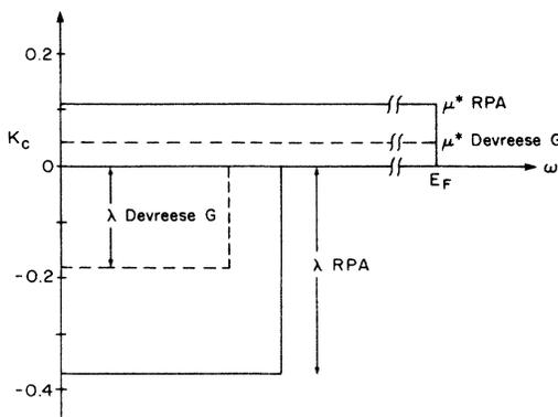
FIG. 7. Two-square-well approximation to the Eliashberg kernel  $K_c(\omega)$  is shown in the RPA by solid lines. By comparison the exchange function Devreese  $G(q)$  reduces the Coulomb interactions and simultaneously lowers the electron repulsion  $\mu^*$  as well as the magnitude of the electron-phonon coupling  $\lambda$ . The net reduction results in exceedingly small values of  $T_c < 0.1$  K. Here the valency was chosen as  $z = 1$ ,  $r_s = 3$ , and the ion mass is  $M = 86$ .
