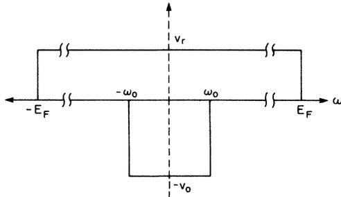
FIG. 4. Schematic representation of the two-square-well model used to approximate the kernel  $K_c(\omega)$  which enters the Eliashberg equations. The model yields an analytic solution for  $T_c(V_0, V_R, \omega_0, E_F)$ , and the various parameters  $V_0, V_R, \omega$  are determined by direct numerical evaluation of kernel  $K_c(\omega)$ .
