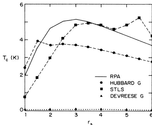
FIG. 5. Computed superconducting transition temperatures are shown as a function of  $r_s$  using  $z=1$  and  $M=86$ . The RPA greatly overestimates  $T_c$  for the nonsuperconducting alkali metals Na, K, Rb, and Cs. The Hubbard and STLS forms of the exchange function  $G(q)$  modify  $T_c$  considerably as shown, but the  $G(q)$  function with a peak near  $q \approx 2k_F$  (Devreese case) dramatically lowers  $T_c$  to values below 0.1 K.
