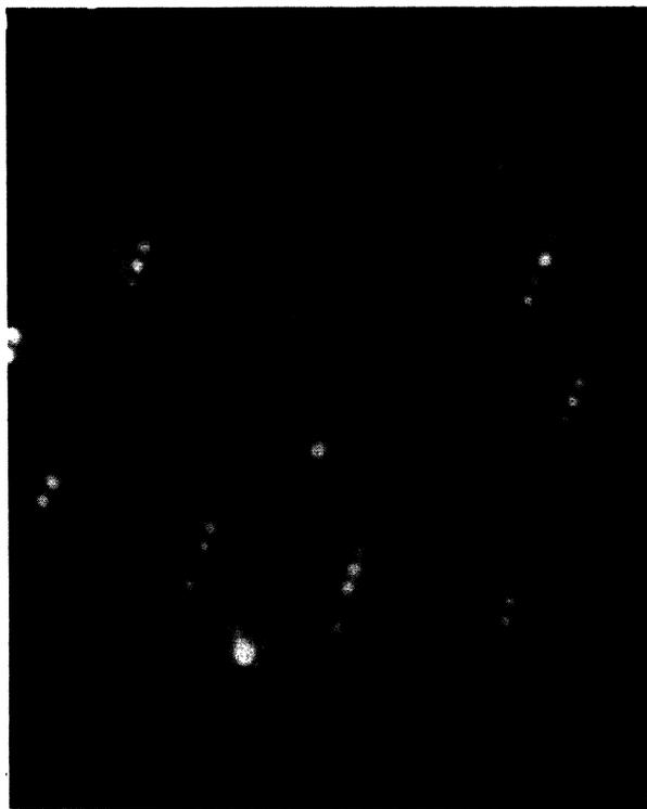
FIG. 1. Display LEED image of an incommensurate Pd monolayer on Ta(110) taken using 128-eV energy primary electrons. Satellite spots attributed to multiple scattering between the overlayer and the substrate are clearly visible.
