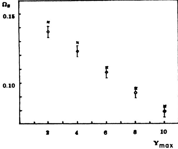
FIG. 1. Kink oscillations frequency  $\Omega_S$  vs  $y_{\max}$ . The parameters are  $\kappa=0.09$ ,  $\alpha=0$ ,  $\epsilon=0$ . The numerical points are represented by circles ( $\circ$ ) with a  $\Delta\Omega_S = \pm 4 \times 10^{-3}$ . The theoretical points given by (23d) and (23e) are represented by crosses ( $\times$ ).  $\Omega_N=0.15$ .
