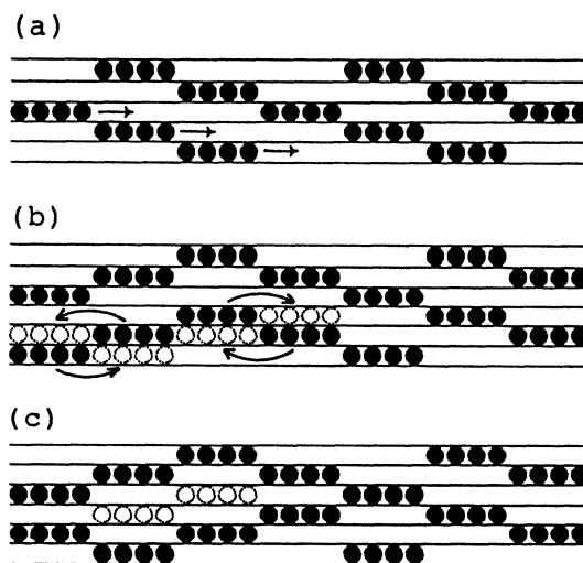
FIG. 1. Three types of intercalation processes are introduced in the present model. (a) Daumas-Hérold domain model for stage-3 structure. Arrows indicate a simultaneous lateral translation of a slanting array of islands. (b) Simultaneous shunting motion of islands shown by the arrows and dotted circles. (c) Growth process of islands shown by dotted circles, which produces two neighboring stage-2 units from the stage-4 unit.
