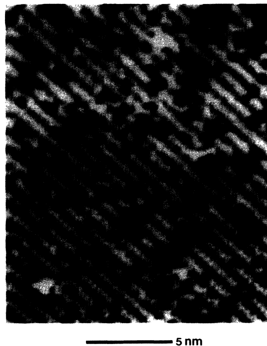
FIG. 5. Large-area topograph of the Si(001) surface illustrating the high density of vacancy-type defects. The gray scale corresponds to a distance change of 1.0 Å.
