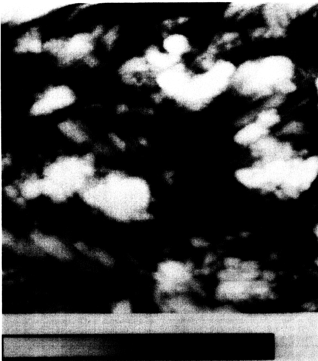
FIG. 16. Gray-scale image of a Si(001) surface which has been annealed to 1450 K and shows faceting. The facets appear as alternating bands at 45^\circ with respect to the axes. The total gray-scale range is 75 \text{ \AA} over the 1000 \times 1000 \text{ \AA} area.
