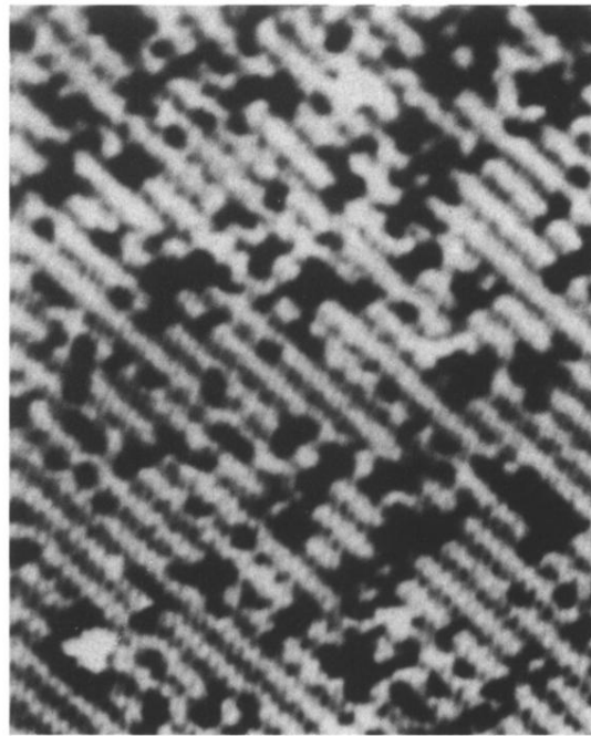
FIG. 5. Large-area topograph of the Si(001) surface illustrating the high density of vacancy-type defects. The gray scale corresponds to a distance change of 1.0 Å.
