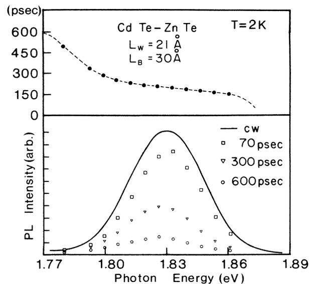
FIG. 1. Continuous-wave and time-resolved exciton recombination spectra from the CdTe-ZnTe superlattice discussed in text (lower panel). The upper panel shows the exciton lifetime in the range of localized states.
