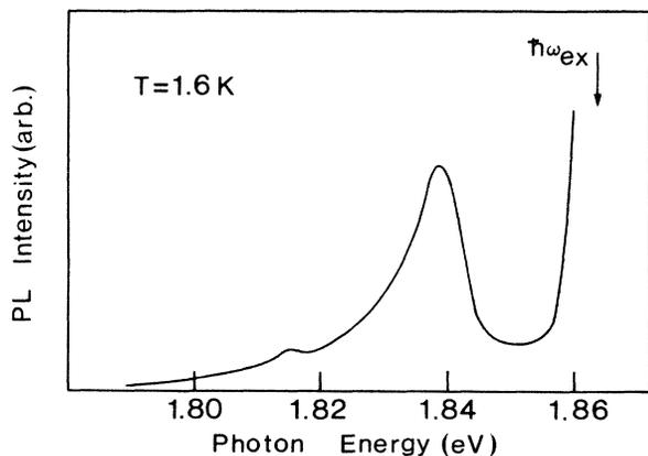
FIG. 2. Luminescence from the CdTe-ZnTe superlattice sample under photoexcitation directly into the localized states (at  $\hbar\omega_{ex} = 1.865$  eV). The sidebands are due to optical-phonon-assisted processes.
