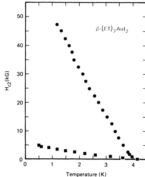
FIG. 3. Temperature dependence of the upper critical field  $H_{c2}$ , as determined from the ac susceptibility of  $\beta\text{-(ET)}_2\text{AuI}_2$ , for fields applied perpendicular to the  $a$ - $b$  plane ( $\square$ ) and parallel to the  $a$  axis ( $\circ$ ).
