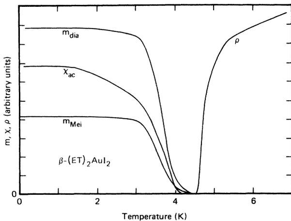
FIG. 2. Various superconducting transition curves of  $\beta\text{-(ET)}_2\text{AuI}_2$ : Diamagnetic shielding  $m_{\text{dia}}$  and Meissner magnetization,  $m_{\text{Meissner}}$  were taken in an applied field,  $H_{\perp ab} = 100$  mG; ac susceptibility  $\chi_{\text{ac}}$  and resistivity  $\rho$ , were taken on the same sample in successive runs in zero magnetic field.
