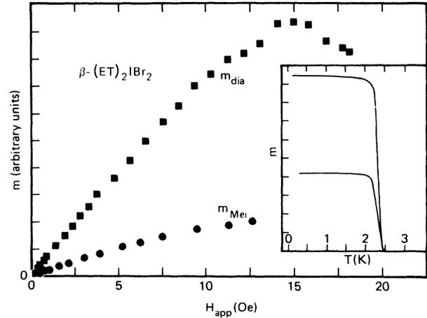
FIG. 1. Magnetization curves of the diamagnetic shielding ( $m_{dia}$ ) and Meissner signal ( $m_{Meissner}$ ) versus applied field ( $\perp a$ - $b$  plane) at  $T = 0.5$  K of  $\beta$ -(ET)<sub>2</sub>IBr<sub>2</sub>. The inset shows the temperature dependence of the diamagnetic shielding and Meissner magnetization in an applied field of  $H_{\perp ab} = 100$  mOe.
