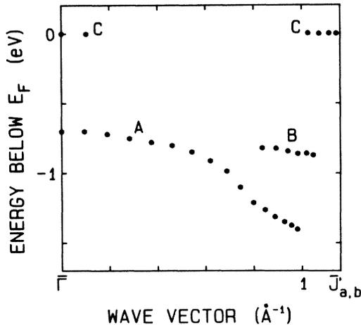
FIG. 3. Initial-state energy dispersions for the surface states *A*, *B*, and *C* along the [010] azimuthal direction.
