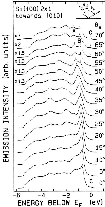
FIG. 1. Photoemission spectra recorded with 10.2-eV photon energy for various angles of emission along the [010] azimuthal direction. The angle of incidence is  $\theta_i = 45^\circ$  except for  $\theta_e = 45^\circ$  and  $50^\circ$  for which  $\theta_i = 55^\circ$ .
