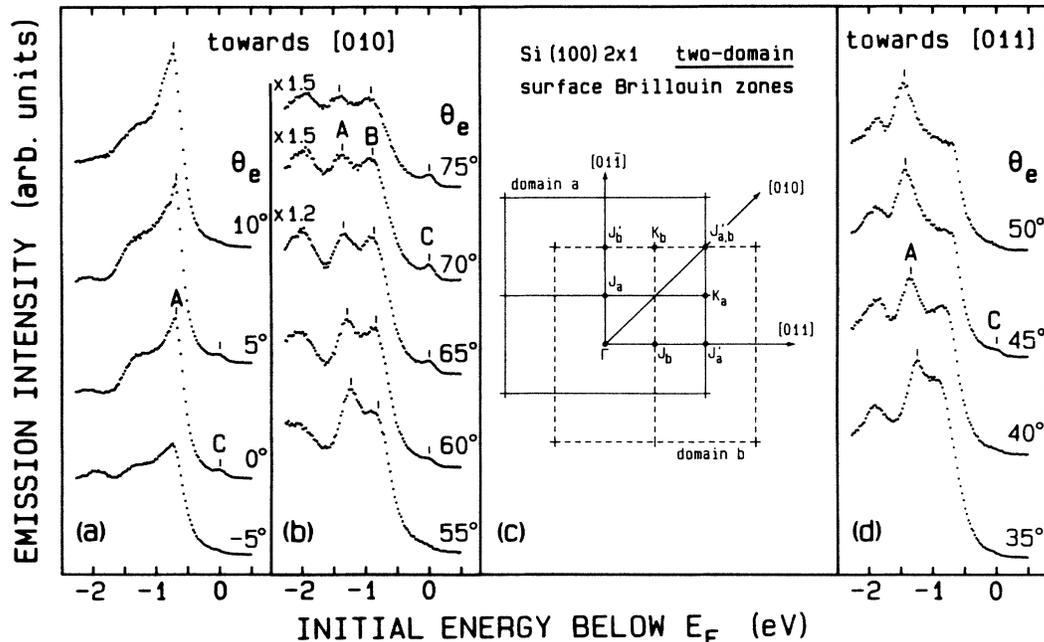
FIG. 2. (a) and (b) Photoemission spectra recorded for various emission angles along the [010] azimuthal direction.  $\theta_i = 45^\circ$ . (c) Superposed surface Brillouin zones of the two different  $2 \times 1$  domains in the repeated zone scheme. (d) Photoemission spectra recorded for various emission angles along the [011] azimuthal direction.  $\theta_i = 45^\circ$  for  $\theta_e = 35^\circ, 40^\circ$ , and  $\theta_i = 55^\circ$  for  $\theta_e = 45^\circ, 50^\circ$ .
