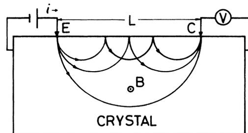
FIG. 1. Experimental setup of the TEF experiment. Electrons are injected through a point contact  $E$  and focused on another point contact  $C$  by means of a uniform magnetic field  $B$ . The electrons can also be focused on  $C$  after one or more specular reflections from the crystal surface. The point-contact distance  $L$  ranges from 50 to 500  $\mu\text{m}$ , the injection current  $i$  is 300 mA, and the collector voltage  $V$  is 0.1 to 800 nV.
