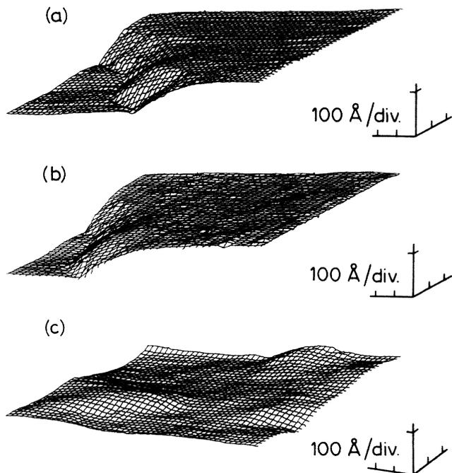
FIG. 3. STM mapping of (a) a Ag(001) surface of  $1450 \times 1300 \text{ \AA}^2$  showing atomically flat regions separated by a large step (approximately  $50 \text{ \AA}$ ), (b) the same area scanned in a direction perpendicular to the previous one, (c) a Ag(011) surface of  $1450 \times 1300 \text{ \AA}^2$  showing a smoothly varying structure. Note the different scales used for the in-plane and out-of-plane axes.
