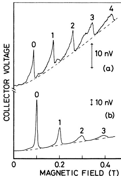
FIG. 2. Reflection measurements with TEF. Clearly, the peaks caused by direct electron focusing (0) and those caused by focusing after one or more reflections from the surface (1, 2, ...) can be seen. The dashed lines indicate the estimated background signal. (a) result from Ag(001),  $\mathbf{B} \parallel [100]$ ,  $L = 150 \mu\text{m}$ ; (b) result from Ag(011),  $\mathbf{B} \parallel [111]$ ,  $L = 200 \mu\text{m}$ .
