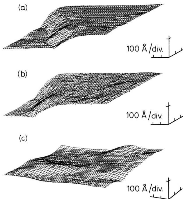
FIG. 3. STM mapping of (a) a Ag(001) surface of  $1450 \times 1300 \text{ \AA}^2$  showing atomically flat regions separated by a large step (approximately  $50 \text{ \AA}$ ), (b) the same area scanned in a direction perpendicular to the previous one, (c) a Ag(011) surface of  $1450 \times 1300 \text{ \AA}^2$  showing a smoothly varying structure. Note the different scales used for the in-plane and out-of-plane axes.
