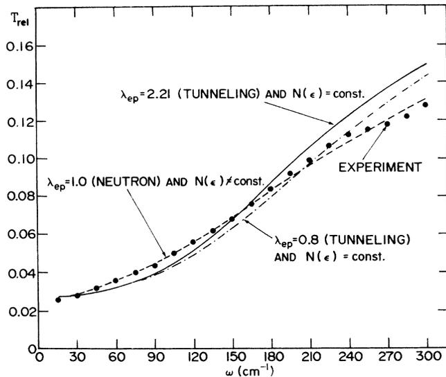
FIG. 3. Calculated and experimental relative transmission  $T_{rel}(\omega)$  in the far infrared of a thin  $V_3Si$  film.  $\omega$  is the radiation frequency (in  $cm^{-1}$ ).
