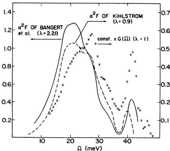
FIG. 1. Tunneling  $\alpha^2F$ 's of Bangert *et al.* (Ref. 1) (solid line) and of Kihlstrom (Ref. 2) (dashed line). The crosses give  $\text{const} \times G(\Omega)$ .
