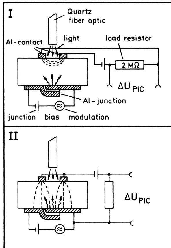
FIG. 1. Different contact configurations for PIC measurements. In case II the bias at the Al contact could be positive (II+) or negative (II-). All samples are bulk doped and the sample thickness is about 3 mm. The measuring temperature was 1.0 K.
