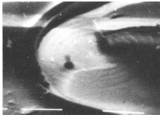
FIG. 1. A typical set of four concentric rings observed on the flaked surface of a blister. (Dose: 8 \times 10^{15} H^+ ions/cm 2 at 250 keV.) (Bar: 10 \mu m.)
