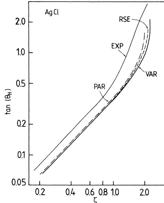
FIG. 5. Field dependence of the tangent of the Hall angle for  $\alpha=1.84$  and for the same  $E(k)$  relations as in Fig. 3. Also indicated are experimental values from Komiyama *et al.* for AgCl for sample M1CB at a fixed electric field of 3.3 kV/cm.
