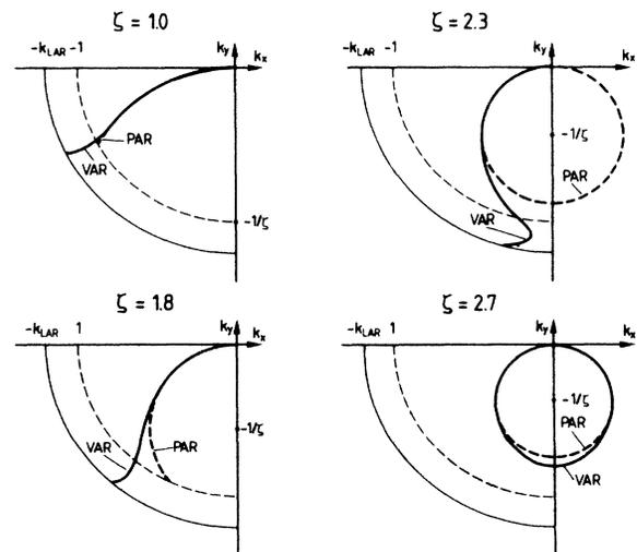
FIG. 3. Solution of the electron equation of motion in  $k$  space for the following two different  $E(k)$  relations: (i) free electron with effective mass (PAR) (thick dashed curve) and (ii) variational calculation of Larsen (VAR) (thick solid curve), and for different values of the dimensionless field.
