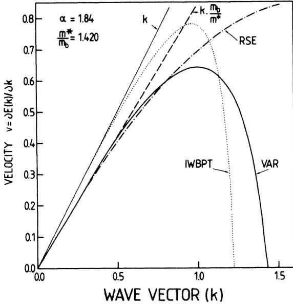
FIG. 2. Wave-vector dependence of the polaron velocity as obtained from the following different theories: (i) free electron with bare band mass (thin solid curve), (ii) free electron with effective mass (dashed curve), (iii) expansion of the Rayleigh-Schrödinger perturbation theory (dashed-dotted curve), (iv) variational calculation of Larsen (VAR) (Ref. 2) (thick solid curve), and (v) IWBPT (dotted curve).
