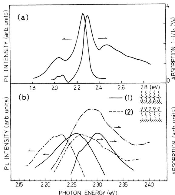
FIG. 1. (a) Absorption and photoluminescence spectra of a PDA monolayer on a hydrophilic glass surface. (b) Exciton peaks of absorption and photoluminescence of a PDA monolayer on a hydrophilic glass surface (inset 1) and on a hydrophobic surface (inset 2). In the inset, circles stand for the hydrophilic head group while the wiggly lines for the alkyl chains. The dot and chain curve is for a tail-to-tail bilayer.
