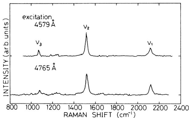
FIG. 3. Resonance Raman spectra of a PDA monolayer at two laser excitation wavelengths. Slowly varying fluorescence background is subtracted.
