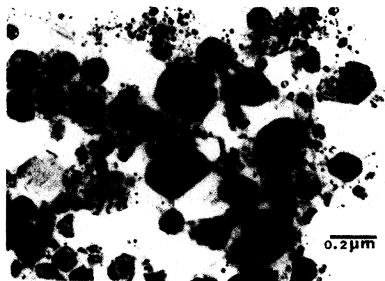
FIG. 3. Transmission electron micrographs of 30% Ni in an MgO sample.
