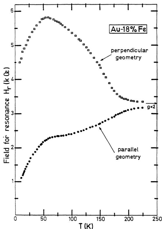
FIG. 2. X-band resonance field  $H_r$  as a function of temperature for plate-shaped sample in parallel and perpendicular field geometry.
