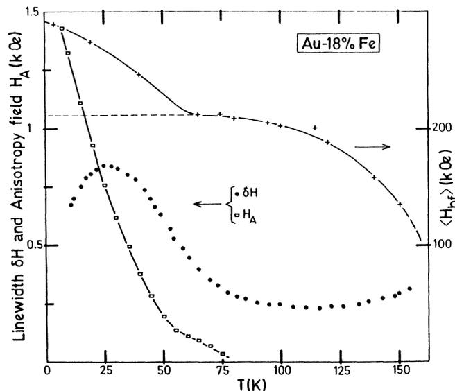
FIG. 3. Temperature variation of the resonance linewidth  $\delta H$  ( $\bullet$ ) and of the deduced anisotropy field  $H_A$  ( $\square$ ) compared with  $^{57}\text{Fe}$  average hyperfine field taken from Ref. 4.
