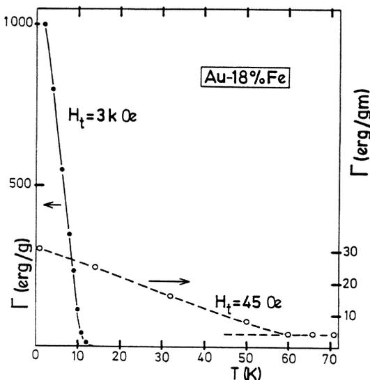
FIG. 1. Torque  $\Gamma$  measured 1 sec after turning magnet through  $5^\circ$  in turning fields  $H_t$  of 3 kOe and 45 Oe.
