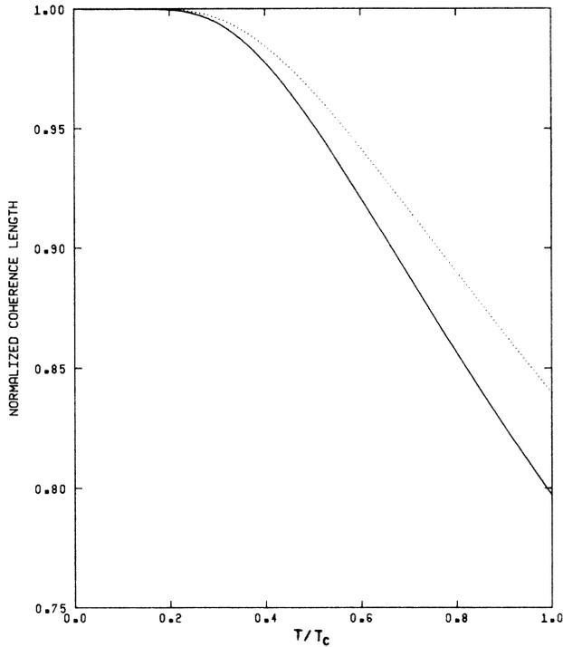
FIG. 1. The coherence length normalized with respect to its zero-temperature value as a function of temperature normalized with respect to the superconducting critical temperature. The material is  $V_3Si$ . The solid curve is the pure case ( $l = \infty$ ); the dotted curve is the slightly dirty case ( $l = 28.0$  nm).
