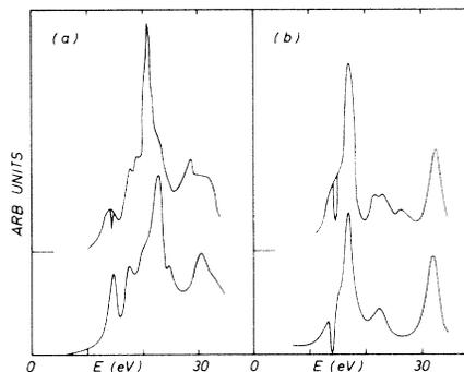
FIG. 4. Upper curves give the  $p$ -projected densities of states as derived from the band-structure calculation. Lower curves give the transition rates as calculated in the cluster model. In (a) the origin is at the Mg site, in (b) at the O site. Both approaches use phase shifts up to  $l = 2$ . Damping is  $-0.5$  eV.
