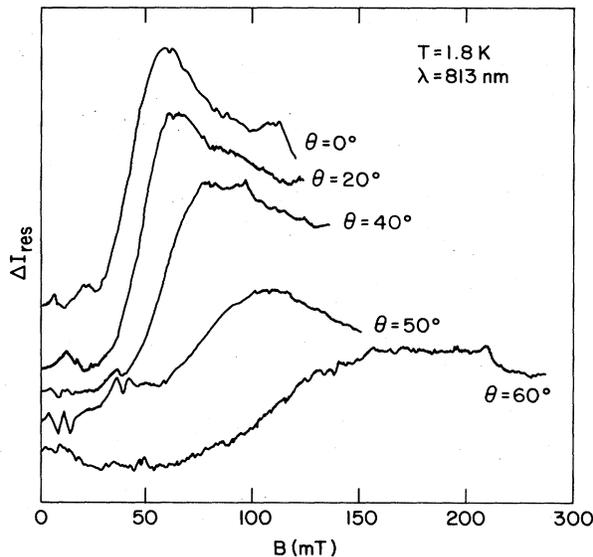
FIG. 2. ODCR for different angles  $\theta$  between the magnetic field and the normal to the MQW layers.
