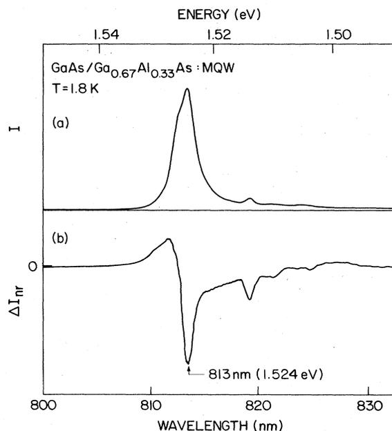
FIG. 1. (a) Luminescence intensity as a function of wavelength. (b) Nonresonant microwave-induced change in luminescence with no applied magnetic field.
