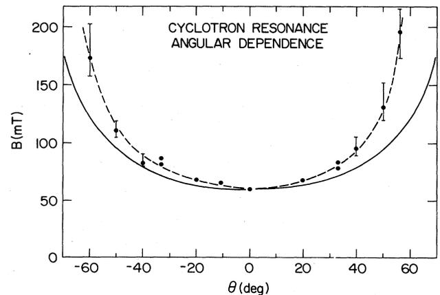
FIG. 3. Angular dependence of the cyclotron resonance peak position. Solid curve is calculated based on a  $\cos\theta$  dependence.
