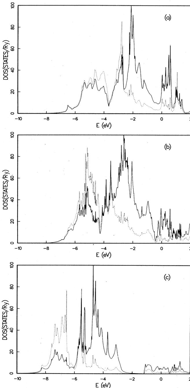
FIG. 3. The  $5d_{3/2}$  (dotted) and  $5d_{5/2}$  (solid) DOS functions in (a)  $\text{UIr}_3$ , (b)  $\text{UPt}_3$ , and (c)  $\text{UAu}_3$ . The zero of energy is at  $E_F$  in each material.
