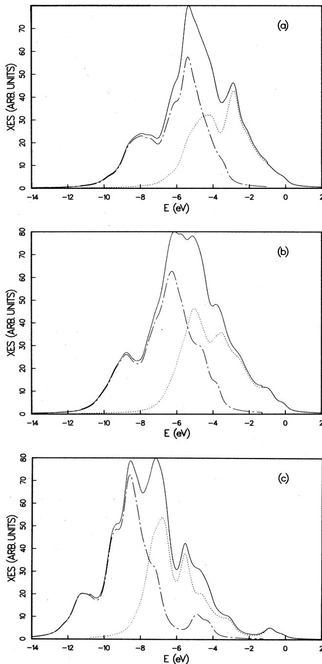
FIG. 1. Theoretical  $N_{6,7}$  spectra for (a) Ir, (b) Pt, and (c) Au in  $\text{UIr}_3$ ,  $\text{UPt}_3$ , and  $\text{UAu}_3$ . The full curves correspond to the superposition of the  $N_7$  (short-dash-long-dash) and  $N_6$  (dotted) spectra. The zero of energy for each material corresponds to the energy cut-off at  $E_F$ . All spectra have 0.5-eV Lorentzian broadening.
