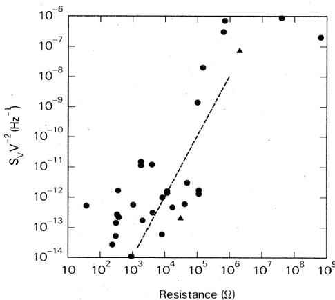
FIG. 2. Normalized  $1/f$  noise  $S_V/V^2$  (or  $S_I/I^2$ ) vs sample resistance for all 31 samples measured. The temperature dependence of the noise is plotted in Fig. 3 for the two samples indicated with triangles. The dashed line is the result of the ion-milling experiment shown in Fig. 4.
