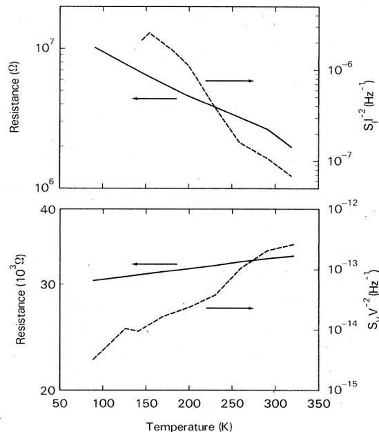
FIG. 3. Resistance and normalized  $1/f$  noise  $S_V/V^2$  (or  $S_I/I^2$ ) for two samples vs temperature. The frequency was 10 Hz. The lower figure is for a metalliclike sample and the upper figure for an insulating sample.
