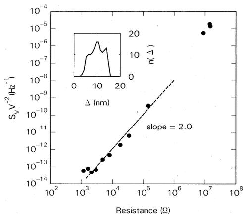
FIG. 4. Normalized  $1/f$  noise  $S_V/V^2$  vs resistance for a single sample measured between ion-milling operations. The frequency was 10 Hz. Inset: Histogram of neck widths in nm for 120 necks measured before ion milling.
