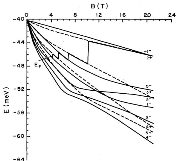
FIG. 2. Landau and Fermi levels with anisotropy effect included.
