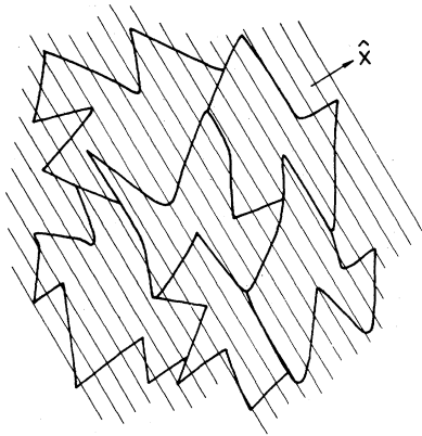
FIG. 25. Orange-peel carpet picture of the amorphous solid. The equicontours of the optical field are superimposed.
