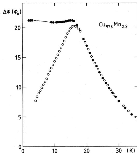
FIG. 1. Magnetic flux changes (in units of a flux quantum  $\phi_0$ ) as monitored by the SQUID magnetometer due to the temperature variation of a  $\text{Cu}_{97.8}\text{Mn}_{2.2}$  bulk sample. The closed circles were obtained by field cooling, the open circles by zero-field cooling (details are given in the text).
