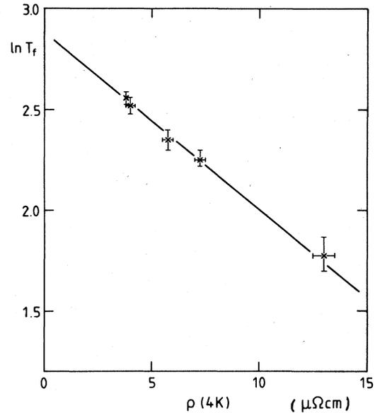
FIG. 5. Logarithmic plot of the spin-glass freezing temperature  $T_f$  as a function of the residual resistivity  $\rho$ . The solid line is obtained by a least-squares fit to the data.
