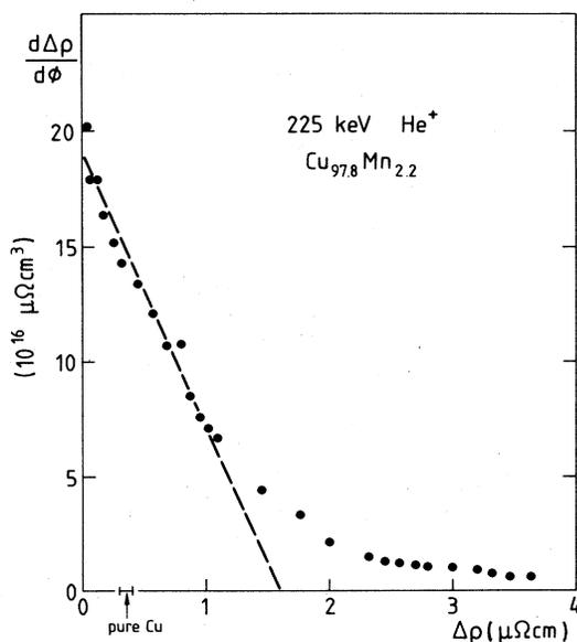
FIG. 2. Damage rate  $d\Delta\rho/d\Phi$  produced in a  $\text{Cu}_{97.8}\text{Mn}_{2.2}$  thin-film spin glass by low-temperature ( $T < 10$  K) He bombardment as a function of the corresponding resistivity increase  $\Delta\rho$  ( $\Phi$  stands for the He fluence). The linear part is indicated by the dashed line.
