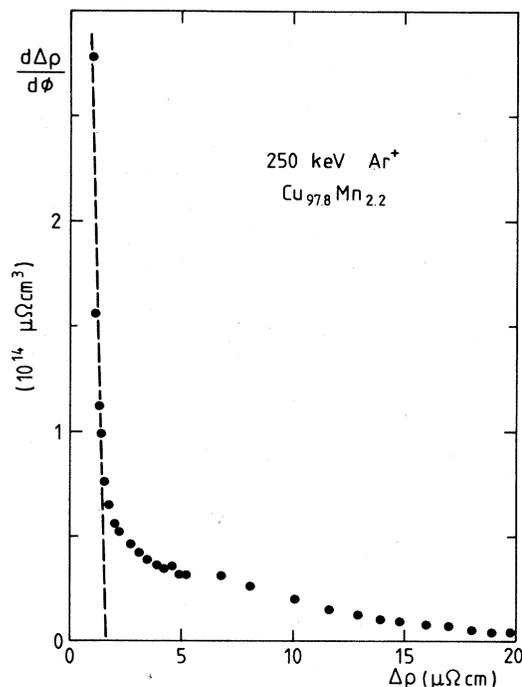
FIG. 3. Damage rate  $d\Delta\rho/d\Phi$  produced in a  $\text{Cu}_{97.8}\text{Mn}_{2.2}$  thin-film spin glass by low-temperature ( $T < 10$  K) Ar bombardment as a function of the corresponding resistivity increase  $\Delta\rho$ . The linear part is indicated by the dashed line.
