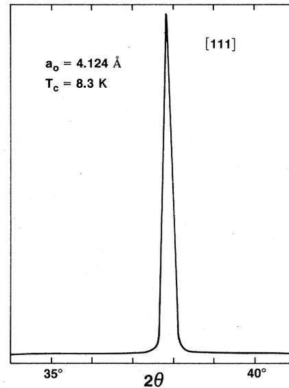
FIG. 1. Typical  $\theta$ - $2\theta$  x-ray diffraction pattern showing the uniaxial growth of the VN films along the [111] direction. The peak height is about 100 times larger than conventional, diode-sputtered films of VN and NbN. No other reflections are observed.
