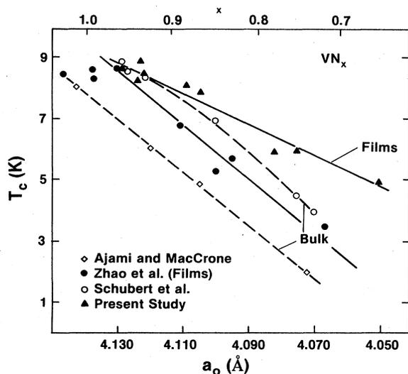
FIG. 2. Superconducting transition temperature  $T_c$  vs lattice parameter  $a_0$  for our films as well as bulk and thin-film results from the literature. The data of Ajami and MacCrone (Ref. 10) are representative of other bulk results. The nitrogen content  $x$  (top abscissa) corresponds with the values of  $a_0$  obtained from the bulk studies. The  $VN_x$  film data point near  $a_0=4.050$  Å was not single phase.
