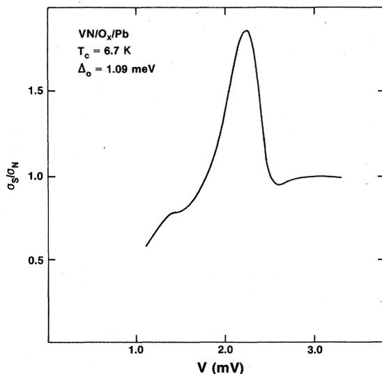
FIG. 5. Normalized dynamic conductance versus bias for VN/O<sub>x</sub>/Pb tunnel junction fabricated by plasma oxidation of the VN surface. A well-defined sum gap is observed leading to the ratio  $2\Delta(0)/k_B T_c = 3.78$ .
