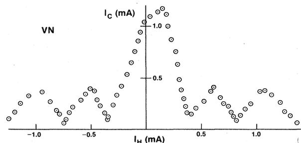
FIG. 6. Maximum Josephson current versus magnet current for a VN tunnel junction utilizing a CdS artificial barrier.
