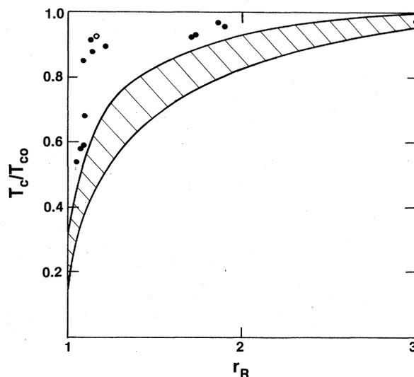
FIG. 3. Superconducting  $T_c$  (normalized  $T_{c0}=9.25$  K) vs resistance ratio  $r_R$  for our  $VN_x$  films. Open circle data point is from the work of Zhao *et al.* (Ref. 7). The shaded region corresponds to the universal behavior demonstrated by high- $T_c$  A15 compounds as well as the ternary compound  $ErRh_4B_4$ . All the  $VN_x$  points lie above the universal curve, clearly demonstrating less sensitivity to disorder.
