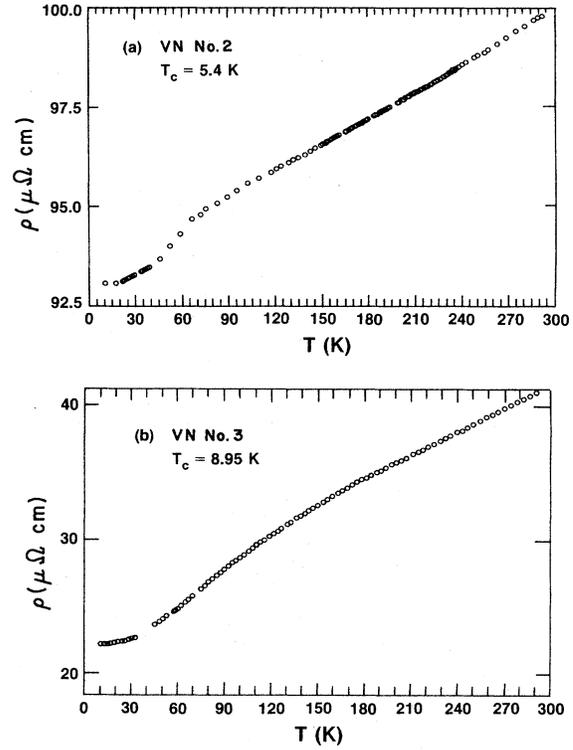
FIG. 4. Resistivity versus temperature for two VN films with resistance ratios (a)  $r_R = 1.07$  for sample 2 and (b)  $r_R = 1.86$  for sample 3.
