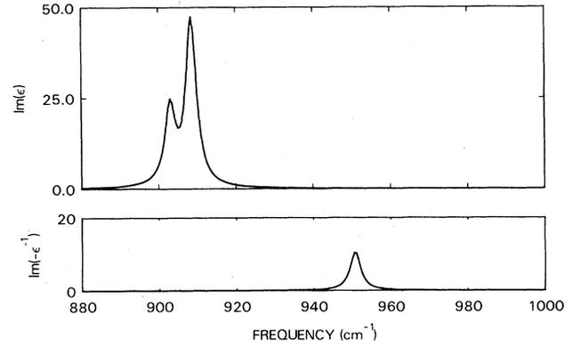
FIG. 2. Resonances of the two mode Lorentz oscillator dielectric function are shown as a function of frequency. In  $\text{Im}(-\epsilon^{-1})$  the double resonance put into  $\epsilon$  has coalesced into a single line.
