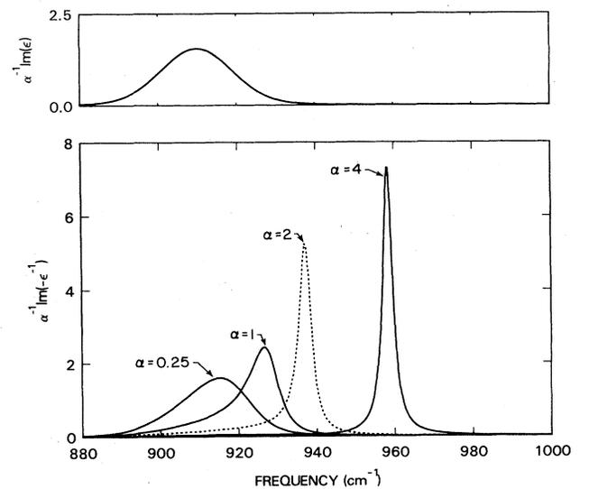
FIG. 3. Resonances of a Gaussian distribution of Lorentz oscillators are shown. The resonance in  $\text{Im}(\epsilon)$  is Gaussian for all  $\alpha$ . In contrast, the resonance in  $\text{Im}(-\epsilon^{-1})$  crosses over from a broad Gaussian to the narrow Lorentzian in the neighborhood of  $\alpha = 1$ , as illustrated.
