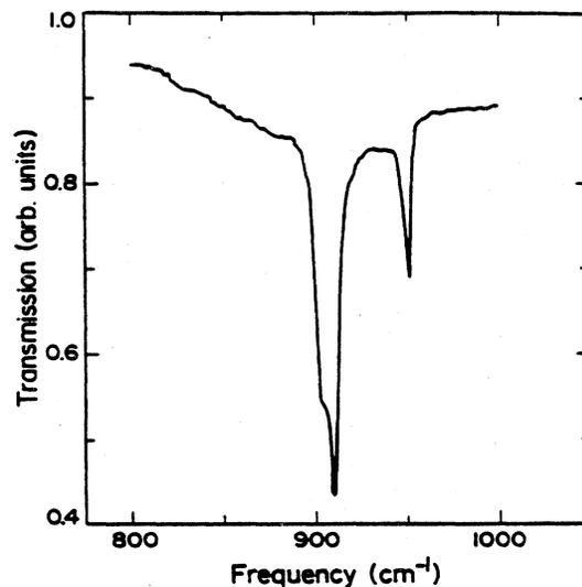
FIG. 1. Absorption lines associated with the  $\nu_3$  mode of  $\text{ReO}_4^-$  in a  $\text{KReO}_4$  film are shown for  $\theta=45^\circ$ . The broad resonance near  $910$   $\text{cm}^{-1}$  is due to oscillations polarized in the film plane, while the sharper and weaker line near  $950$   $\text{cm}^{-1}$  is due to perpendicular oscillations.
