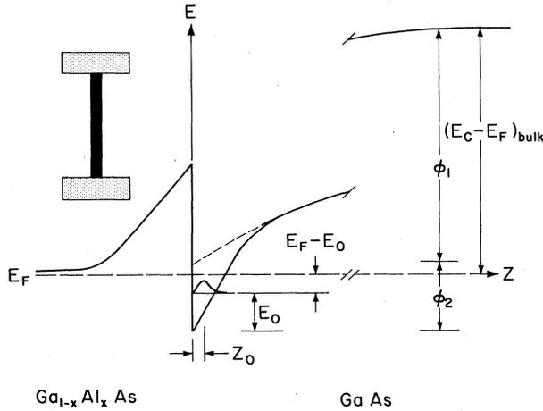
FIG. 1. Schematic diagram of the conduction-band edge for a modulation-doped GaAs-(AlGa)As heterojunction showing the quantities used in the derivation of the relationship between the measured capacitance and the density of states. An outline of the sample geometry is also shown.
