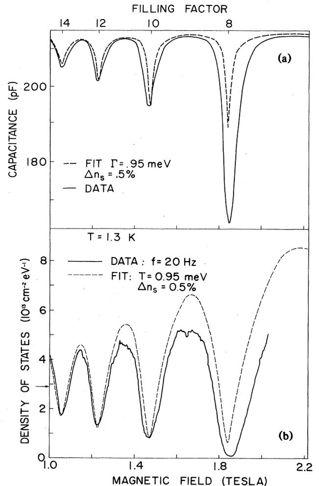
FIG. 3. The measured and calculated capacitance (a) and density of states (b) vs magnetic field. The dashed line is the approximation for  $\nu = 10, 12$ , and 14, based on a model using Gaussian Landau levels. The arrow indicates the zero-magnetic-field density of states.
