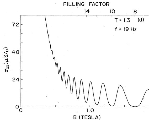
FIG. 2. (a) The magnitude and (b) phase angle of the measured capacitance vs magnetic field. The phase angle is defined so that a purely capacitive signal has a phase angle of  $0^\circ$  and a purely resistive signal has a phase angle of  $90^\circ$ . (c) The density of states determined from the measured capacitance. (d) The conductivity of a circular geometry device fabricated from the same material.
