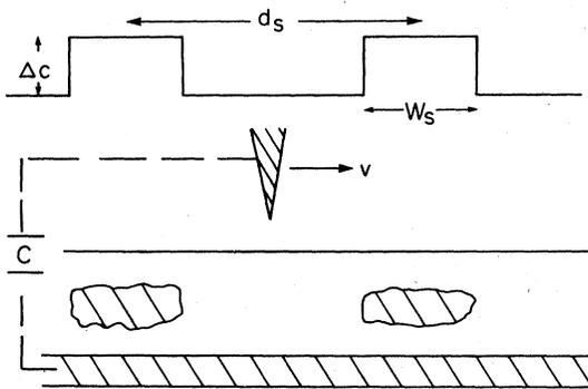
FIG. 1. Schematic illustration of the simple model of the composite system considered in the text and the capacitive pickup response  $\Delta C$  due to the presence of finite conducting clusters of size  $s$ .
