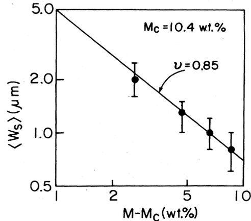
FIG. 3. Dependence of the distance  $\langle w_s \rangle$  on the carbon-black loading,  $M$ . It is shown that the data are consistent with a correlation length type dependence  $(M - M_c)^{-0.85}$ .
