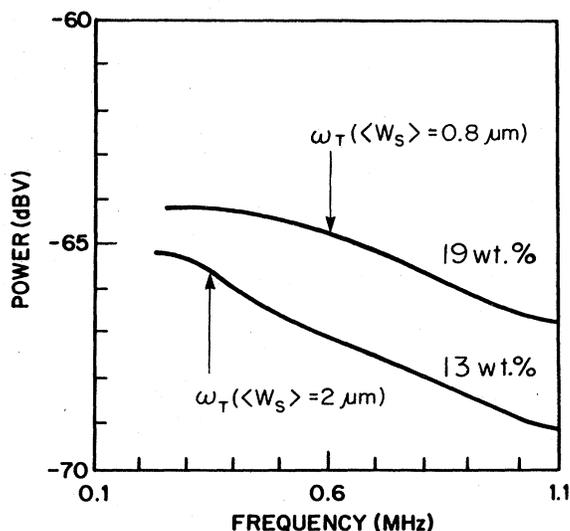
FIG. 2. Power spectra of carbon-black-PVC composites with two different carbon-black loadings. The frequency  $\omega_T$  designates the transition from the low- to the high-frequency regimes. Also indicated is the corresponding distance  $\langle w_s \rangle = 2\pi v / \omega_T$  along the stylus path. (0 dBV = 1 V rms.)
