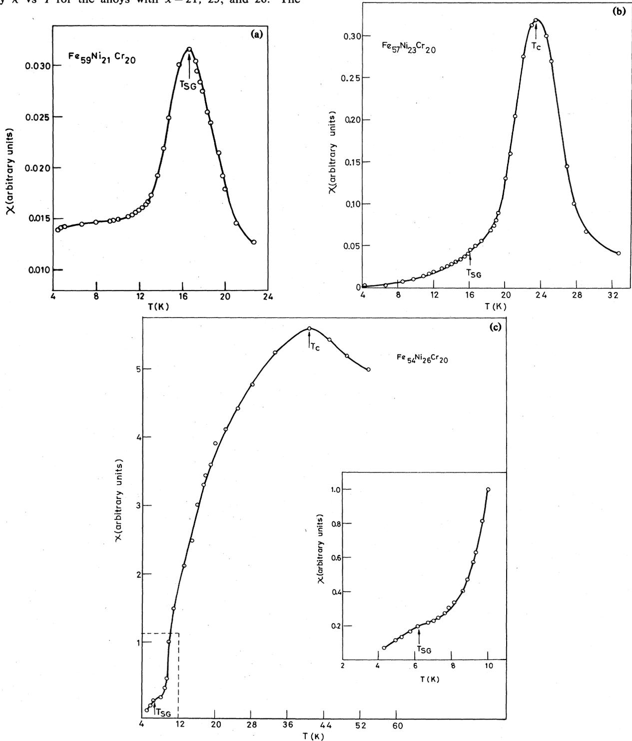
FIG. 1. (a)–(c): ac susceptibility vs temperature for  $\text{Fe}_{80-x}\text{Ni}_x\text{Cr}_{20}$  alloys with  $x=21$ , 23, and 26, respectively.
