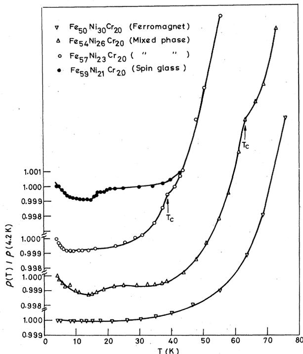
FIG. 2.  $\rho(T)/\rho(4.2 \text{ K})$  vs temperature for  $\text{Fe}_{80-x}\text{Ni}_x\text{Cr}_{20}$  alloys with  $21 \leq x \leq 30$ .
