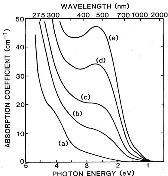
FIG. 1. Optical absorption of  $\text{LiTaO}_3$  measured at 80 K using unpolarized light propagating perpendicular to the  $c$  axis of the sample. Trace (a) represents the as-received crystal, and traces (b), (c), (d), and (e) represent the absorption induced by 1-h reductions in argon at temperatures of 850, 875, 900, and 925 °C, respectively.
