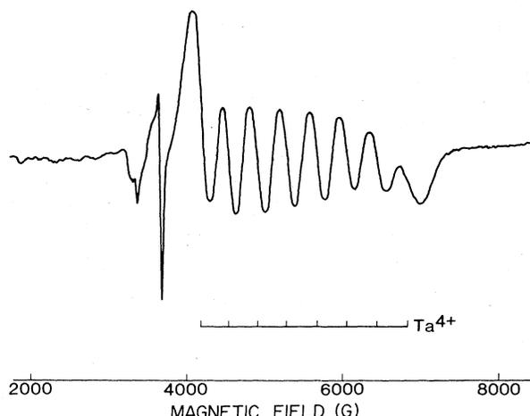
FIG. 3. ESR spectrum of  $Ta^{4+}$  ions in  $LiTaO_3$ . The microwave frequency was 9.449 GHz, the temperature was 17 K, and the magnetic field was oriented perpendicular to the  $c$  axis of the crystal.
