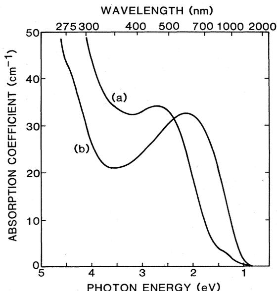
FIG. 2. Effect of a 77-K optical bleach on the optical-absorption spectrum of a  $\text{LiTaO}_3$  crystal that had been reduced for 1 h in argon at 900 °C. Trace (a) was taken before the bleach and trace (b) was taken after the bleach.
