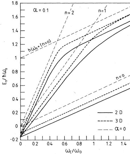
FIG. 1. The first three Landau levels as function of the magnetic field for the unperturbed energy levels (thin dashed curves), the 2D polaron (thick solid curves) and the 3D polaron (thick dashed curves). The electron-phonon coupling constant is  $\alpha=0.1$ .
