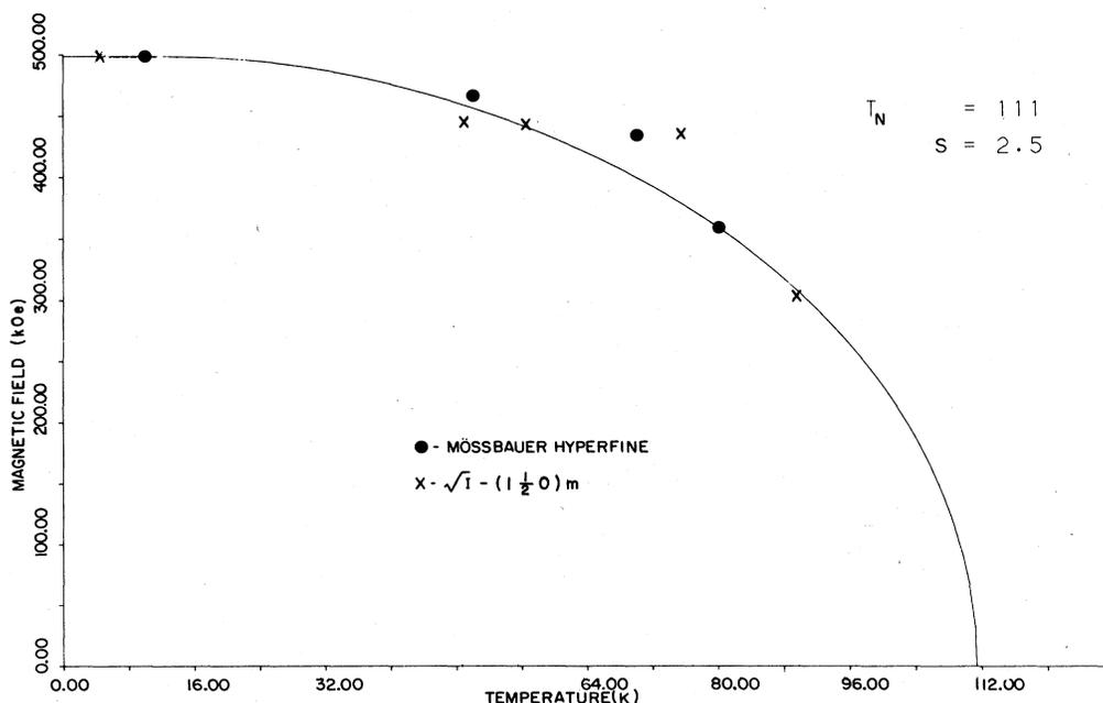
FIG. 8. Mössbauer magnetic hyperfine field (●) for FeOHSO<sub>4</sub> and (x)  $-\sqrt{I}$  against temperature [where  $I$  is the intensity of the  $(1, \frac{1}{2}, 0)$  magnetic reflection of FeOHSO<sub>4</sub> in an  $(a, b, c)$  cell taken from Scheerlinck (Ref. 2)].
