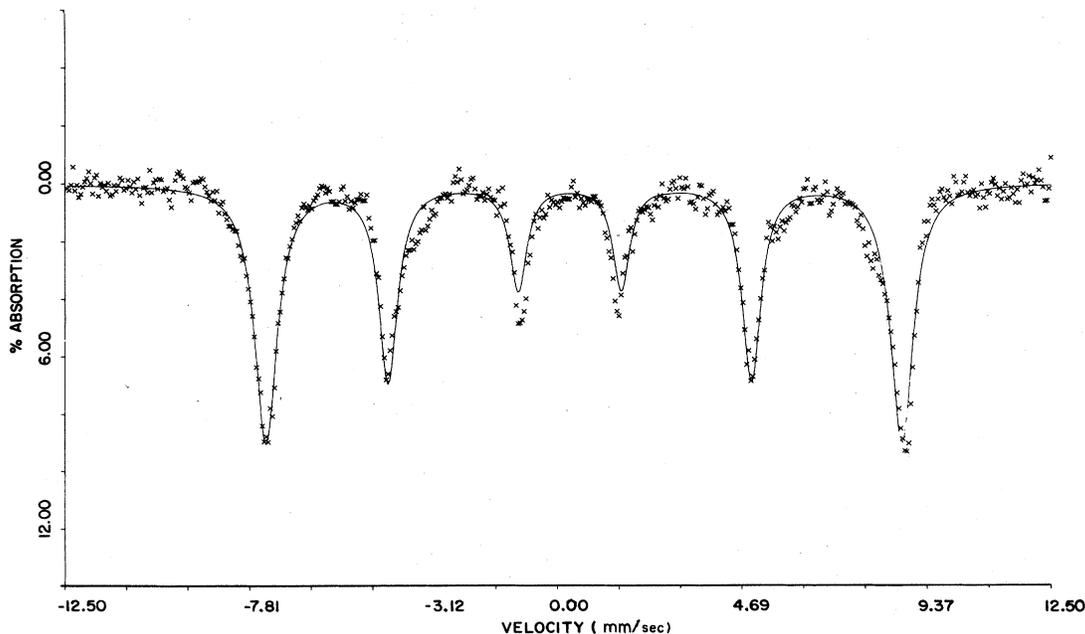
FIG. 4. Mössbauer spectra of  $\text{FeOHSO}_4$  at 4 K.
