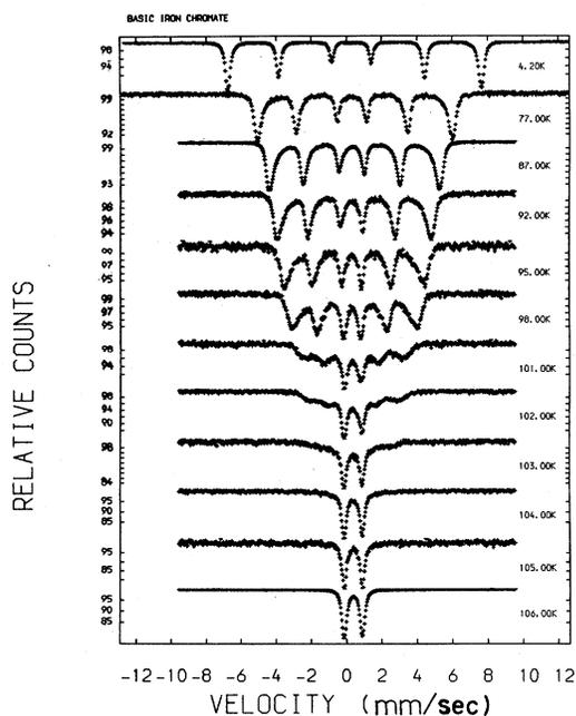
FIG. 5. Mössbauer spectra of  $\text{FeOHCrO}_4$  at various temperatures.
