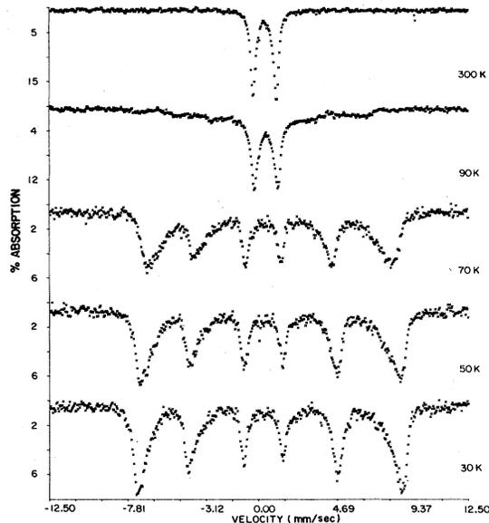
FIG. 3. Mössbauer spectra of  $\text{FeOHSO}_4$  at various temperatures.
