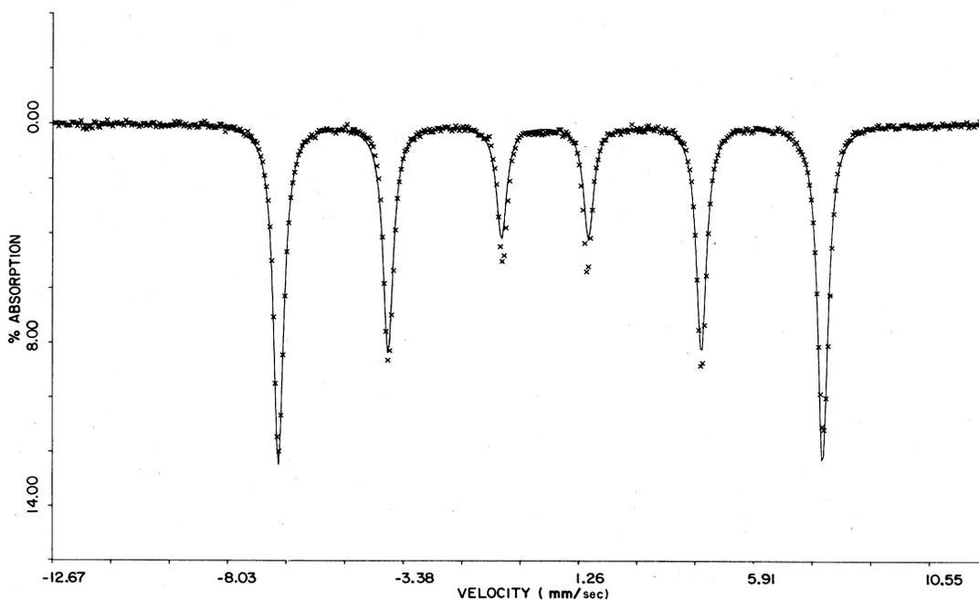
FIG. 6. Mössbauer spectrum of  $\text{FeOHCrO}_4$  at 4 K.
