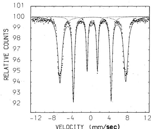
FIG. 7. Mössbauer spectrum of FeOHCrO<sub>4</sub> at 4 K in an external field of 40 kOe.
