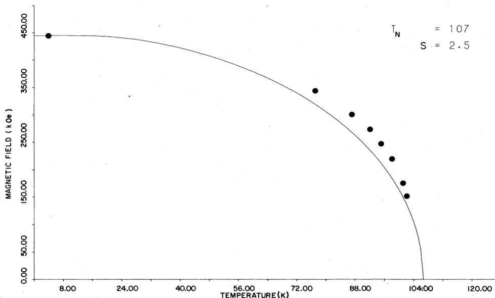
FIG. 9. Mössbauer magnetic hyperfine field of FeOHCrO<sub>4</sub> against temperature.
