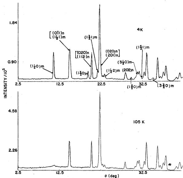
FIG. 2. Neutron-diffraction patterns of  $\text{FeOHCrO}_4$  at 4 and 105 K. The lines are indexed for an orthorhombic cell:  $a = 7.50 \text{ \AA}$ ,  $b = 6.68 \text{ \AA}$ ,  $c = 7.26 \text{ \AA}$  at 4 K.
