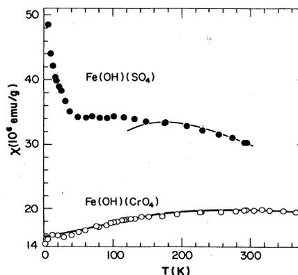
FIG. 1. Magnetic susceptibilities at various temperature for  $\text{FeOHSO}_4$  and  $\text{FeOHCrO}_4$  with fits to experimental data using a Bonner-Fisher, linear-chain model (Refs. 8 and 9).
