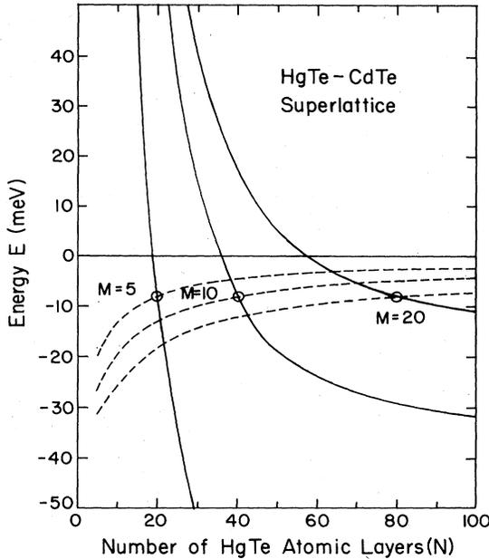
FIG. 2. Energies of interface states with symmetric (dashed) and antisymmetric (solid)  $p$ -component envelope functions calculated in Bastard's model are plotted as functions of the number of HgTe atomic layers ( $N$ ) for fixed number of CdTe atomic layers ( $M=5, 10, \text{ and } 20$ ). The circles indicate the positions where two interface states of opposite symmetries cross.
