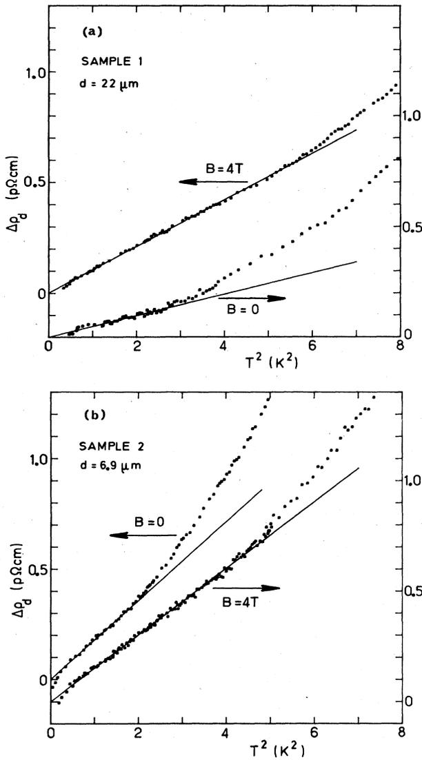
FIG. 1. Temperature-dependent part of the resistivity of the unstrained samples in zero magnetic field and in a longitudinal field of  $B = 4$  T. The straight lines represent fits in the temperature ranges listed in Table I.
