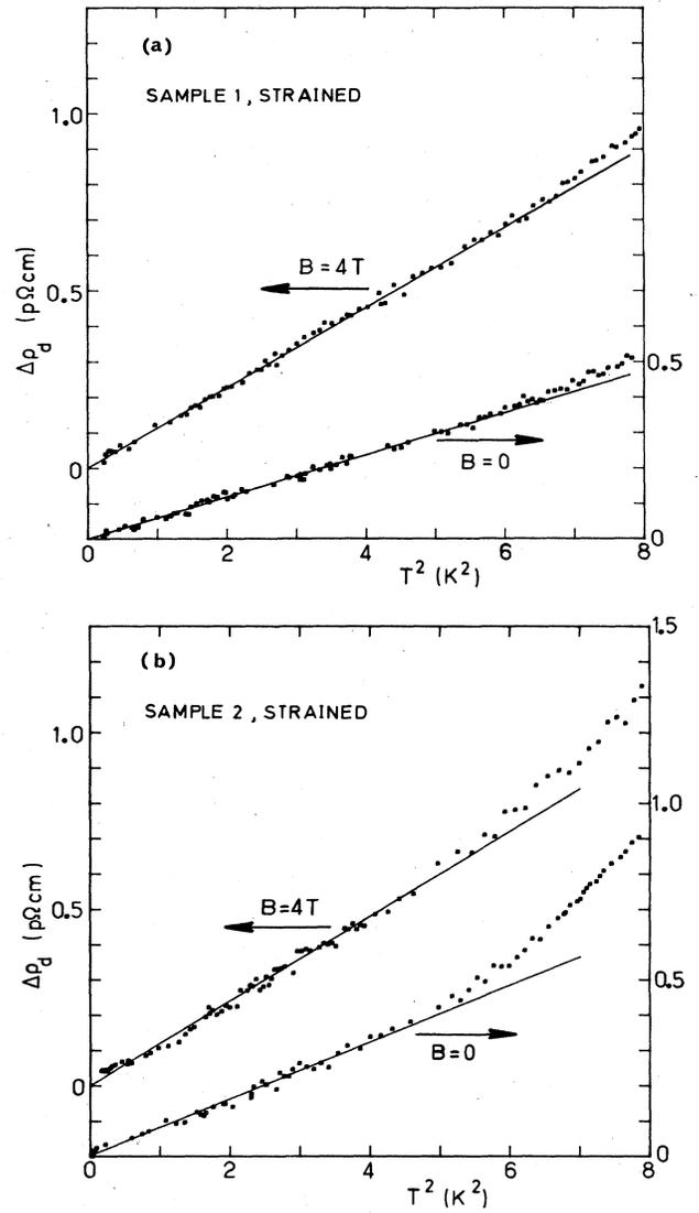
FIG. 2. Effect of straining on the temperature-dependent part of the resistivity of the same samples as in Fig. 1.
