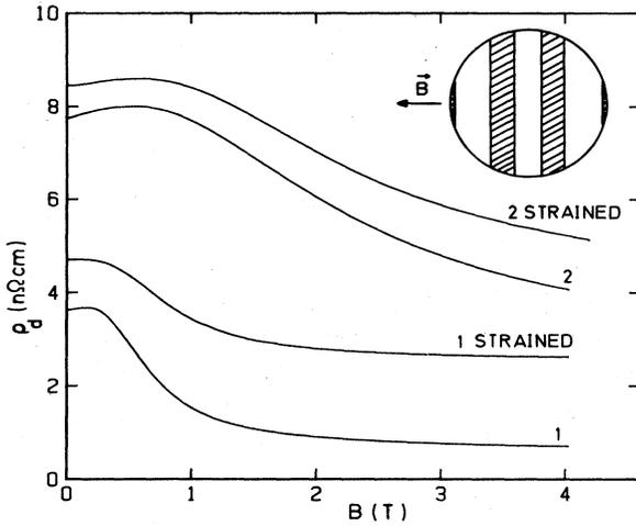
FIG. 3. The longitudinal magnetoresistivity  $\rho_d(B)$  for both samples at  $T=2$  K. Inset: simplified drawing of the Fermi surface of copper for  $\mathbf{B} \parallel (111)$  (see text).
