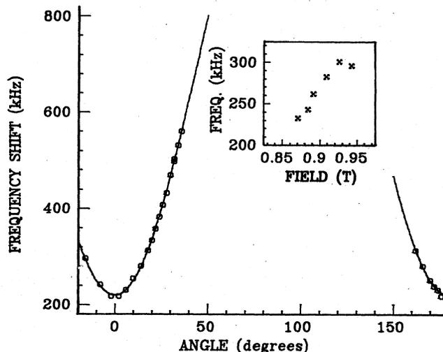
FIG. 3. Frequency shift (relative to bulk <sup>65</sup>Cu) of the 0.1185 MHz/T shifted-Cu line (Fig. 1) as a function of angle. The fit is to the equation  $\Delta f = a_0 + a_2 \cos^2 \theta$ . Inset: The frequency shift, in kHz, of the 0.1185 MHz/T line increases with increasing magnetic field.
