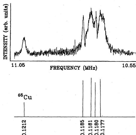
FIG. 1. Typical magnitude spectrum of Cu/Nb, taken at 1.7 K and at  $\theta = -8^\circ$ . The spectrum shows  $^{65}\text{Cu}$ ; it is centered at 10.8 MHz and is 0.5 MHz wide. The numbers across the bottom are the frequencies divided by the field, in units of MHz/T, and serve to identify the lines.
