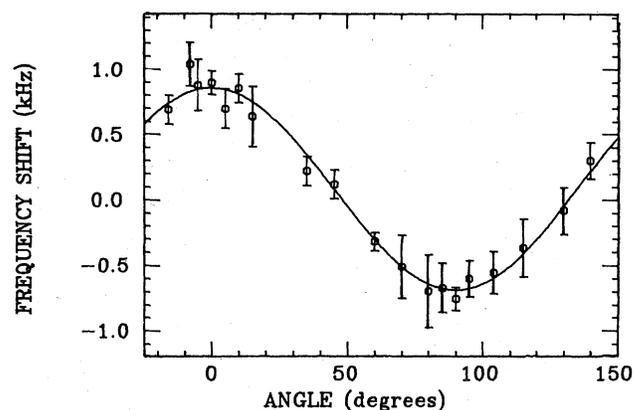
FIG. 2. Frequency shift of Cu/Nb relative to a reference sample of copper powder as a function of angle, corrected for the demagnetization effect. These  $^{65}\text{Cu}$  data were taken at 4.2 K. The fit is to the equation  $\Delta f = a_0 + a_2 \cos^2\theta$ .
