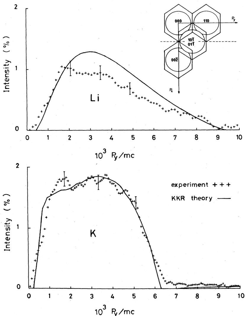
FIG. 3. Profile through the projection of  $(01\bar{1})$  and  $(10\bar{1})$  HMC's as shown in the inset and by the heavy lines in Figs. 1 and 2. Typical statistical errors are shown, but the scatter of points has been reduced by a smoothing procedure. The vertical scale is as in Fig. 1.
