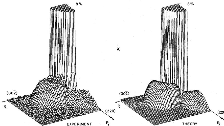
FIG. 2. Higher momentum components of the experimental angular correlation of annihilation photons from K compared with the KKR calculation. The vertical scale is as in Fig. 1.
