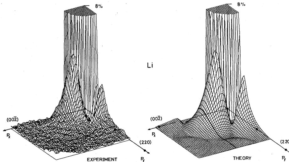
FIG. 1. Higher momentum components of the experimental angular correlation of annihilation photons from Li compared with the KKR calculation. The results are given as a fraction of the conduction-electron contribution at  $p_x = p_y = 0$ .
