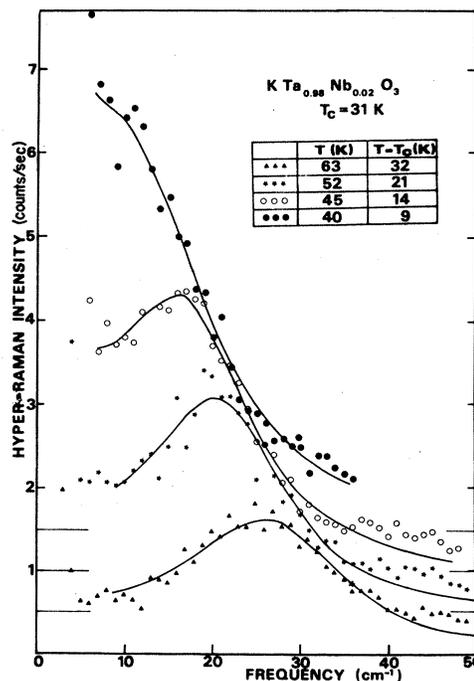
FIG. 4. Hyper-Raman spectra of  $\text{KTa}_{0.98}\text{Nb}_{0.02}\text{O}_3$  between 63 and 40 K. The different spectra have been recorded under the same experimental conditions. Their intensities are given in the same scale. The solid lines represent Lorentzian fits.
