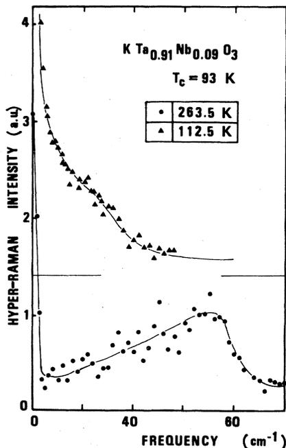
FIG. 7. Hyper-Raman spectra of the ferroelectric soft mode of  $\text{KTa}_{0.91}\text{Nb}_{0.09}\text{O}_3$  at 263.5 and 112.5 K.
