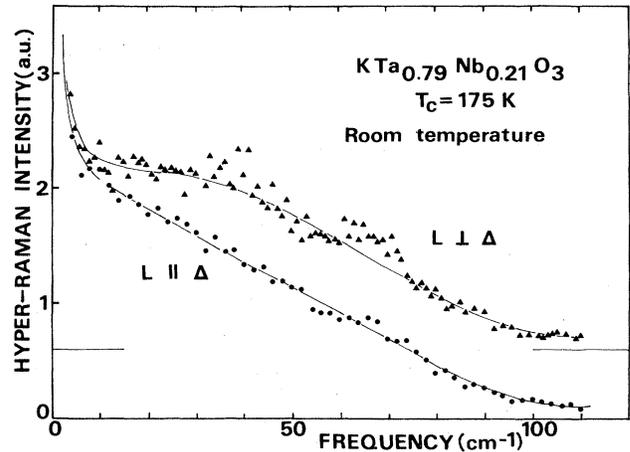
FIG. 8. Hyper-Raman spectra of the ferroelectric soft mode of  $\text{KTa}_{0.79}\text{Nb}_{0.21}\text{O}_3$  at room temperature with the direction of the incident and scattered light parallel and perpendicular to the direction  $\Delta$  of the concentration gradient.
