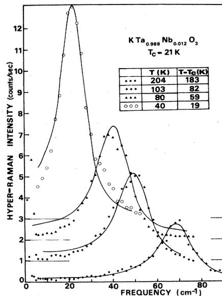
FIG. 3. Hyper-Raman spectra of  $\text{KTa}_{0.988}\text{Nb}_{0.012}\text{O}_3$  at 240, 103, 80, and 40 K. The different spectra have been recorded under the same experimental conditions. Their intensities are given in the same scale. The solid lines represent Lorentzian fits.
