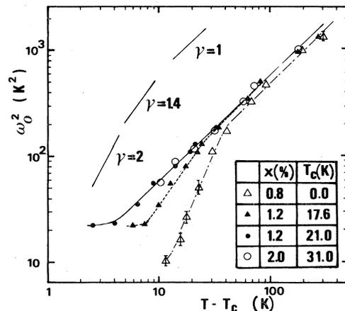
FIG. 6. Double-logarithmic representation of the square of the soft-mode frequency ( $\omega_0^2$ ) as a function of  $T - T_c$  in KTN ( $x=0.008$ ,  $0.012$ , and  $0.02$ ). The crystal with a Nb concentration of  $x=0.012$  is represented with two different  $T_c$  assumptions (solid circles,  $T_c$  as determined from SHG measurements; solid triangles,  $T_c$  as determined from acoustic measurements).
