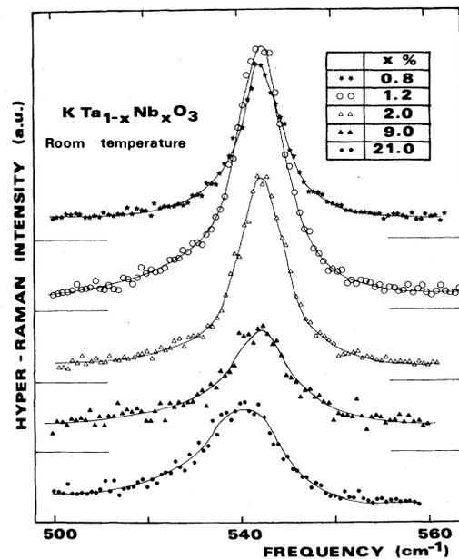
FIG. 9. Hyper-Raman spectra of the TO mode at about  $540 \text{ cm}^{-1}$  at room temperature for the five crystals under investigation.
