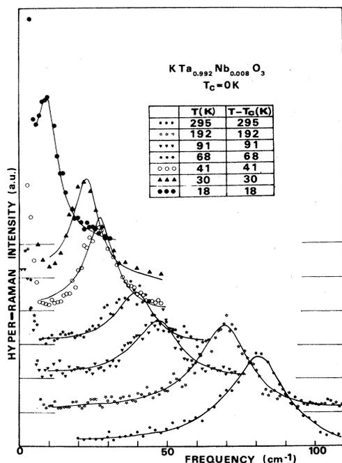
FIG. 2. Typical hyper-Raman spectra of  $\text{KTa}_{0.992}\text{Nb}_{0.008}\text{O}_3$  for various temperatures. Note that the HR intensities for various temperatures are not drawn with the same intensity scale. The solid lines represent Lorentzian fits.
