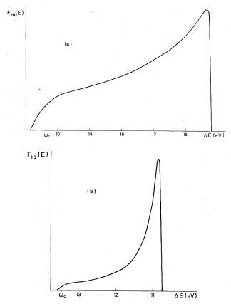
FIG. 4. (a) Shape of the first bulk-plasmon satellite before the convolution with the no-loss line.  $[\omega_c = \omega(k_c).]$  (b) Shape of the first surface-plasmon satellite before the convolution with the no-loss line.
