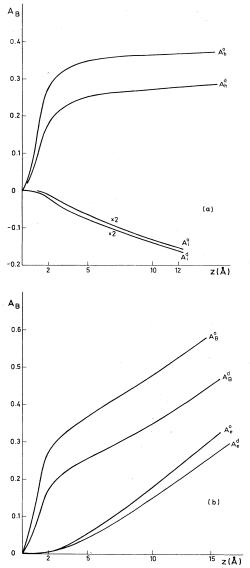
FIG. 2. (a) Intrinsic  $(A_h)$  and interference  $(A_i)$  contributions to the bulk term (2.25) as a function of excitation depth z. Superscripts are as follows: o, the results of the independentplasmon model; d, plasmons with dispersion and damping. (b) Extrinsic contribution  $(A_e)$  and total  $(A_B)$  bulk term.
