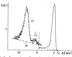
FIG. 5. Comparison of our theoretical results (solid line, in arbitrary units) for  $\lambda = 29$  Å with the experimental results (dots) of Baird *et al.* (Ref. 29) for the XPS spectra from the 2*p* level of Al. Other parameters are the Gaussian half-widths  $\sigma_L = 1.17$  eV and  $\sigma_R = 0.68$  eV, and the background constant C = 0.05 leV.
