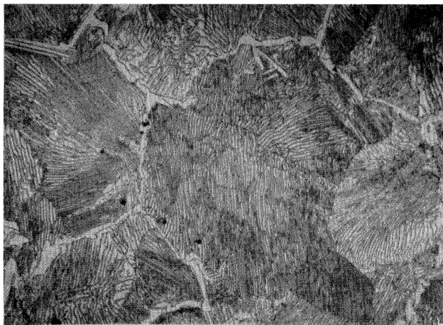
FIG. 3. Isothermal eutectoid colonies in a multicrystalline steel. 10
