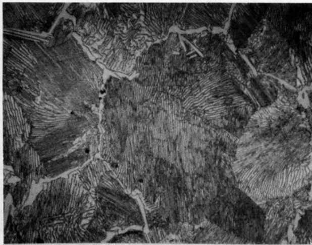
FIG. 3. Isothermal eutectoid colonies in a multigrained steel. 10
