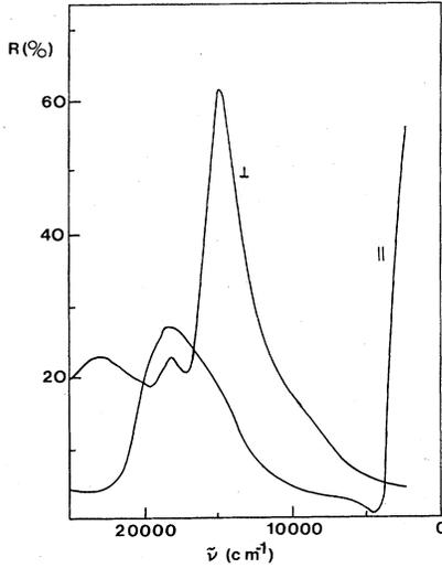
FIG. 1. Room-temperature polarized reflectance spectrum of a single crystal of Ni(pc)I. The perpendicular ( $\perp$ ) orientation has the electric field polarized perpendicular to the highly conducting stacking axis, while the parallel ( $\parallel$ ) orientation has the electric field polarized along the stack axis.
