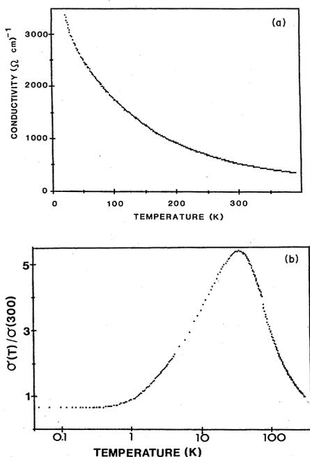
FIG. 2. (a) Temperature dependence of the needle-axis ( $\hat{c}$  axis) conductivity of a Ni(pc)I crystal taken between 20 and 300 K. (b) Temperature dependence of the single-crystal needle-axis conductivity emphasizing the low-temperature behavior; the conductivity has been normalized to an ambient temperature value of about  $450 \Omega^{-1} \text{cm}^{-1}$ .
