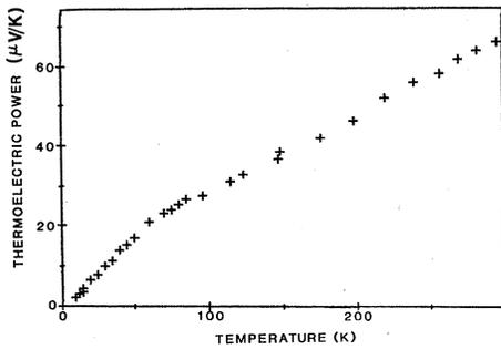
FIG. 3. Temperature dependence of the needle-axis thermoelectric power(s) of a Ni(pc)I crystal taken between 10 and 300 K.
