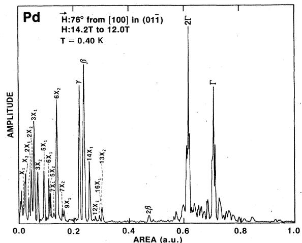
FIG. 3. Fourier spectrum of the frequencies in Pd for the field  $76^\circ$  from [100] in the  $(01\bar{1})$  plane, showing the open hole  $\gamma$  and  $\beta$  frequencies and the interfering harmonics from the  $X$ -centered hole pockets. The second harmonic of the  $\Gamma$ -centered sheet ( $2\Gamma$ ) has been aliased.
