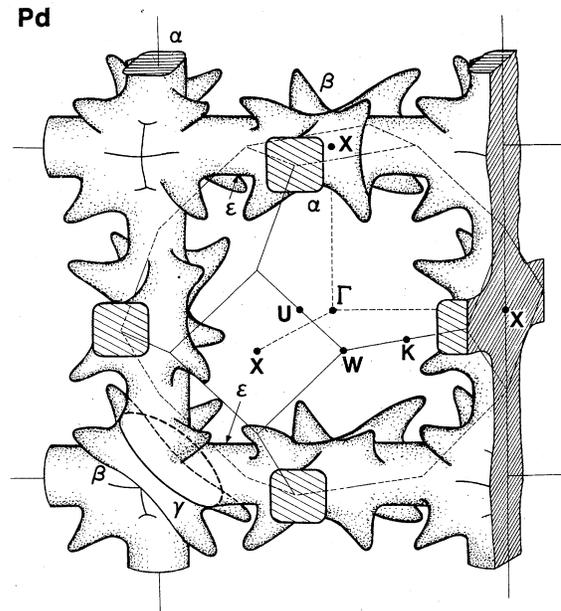
FIG. 1. Fifth-band open hole sheet (scaffolding) of the Fermi surface of Pd [after A. R. Mackintosh and O. K. Anderson, in *Electrons at the Fermi Surface*, edited by M. Springford (Cambridge University Press, Cambridge, 1980), p. 207] showing representative extremal orbits ( $\alpha, \beta, \gamma, \epsilon$ ), the Brillouin zone, and high-symmetry points. The protruding "fins" centered at the  $X$  point contribute strongly to the density of states.
