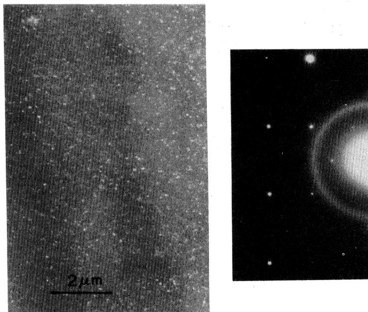
FIG. 10. (a) TEM dark field micrograph of a 100-Å Ti film on atomically clean Si(111) reacted at 300°C for 20 min; (b) corresponding diffraction pattern.
