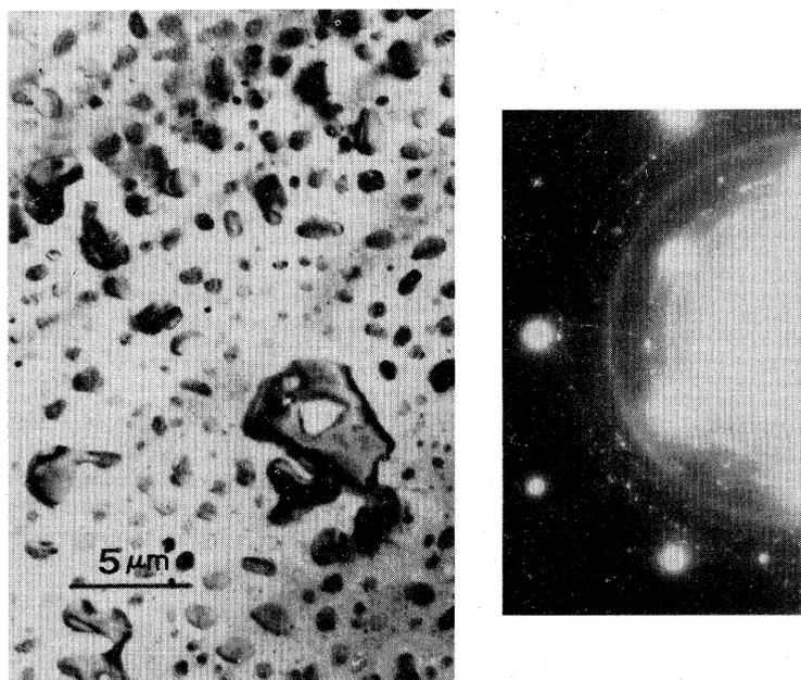
FIG. 11. (a) TEM bright field micrograph of a 100-Å Ti film on atomically clean Si(111) reacted at 300°C for 20 min and then at 780°C for 3.5 h; (b) corresponding diffraction pattern.
