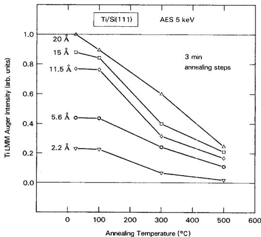
FIG. 2. AES intensity behavior of Ti  $L_{2,3}M_{2,3}M_{2,3}$  as a function of annealing temperature for various coverages. Annealing times were 3 min each.
