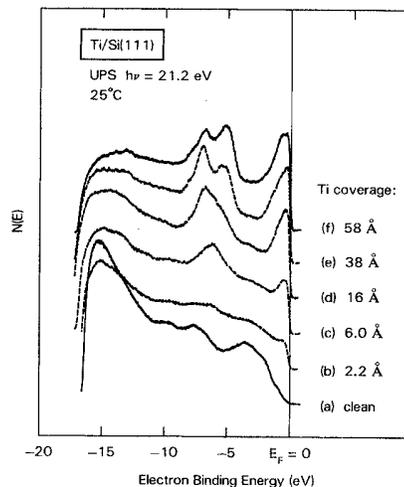
FIG. 3. UPS ( $h\nu = 21.2$  eV) spectra for (a) clean Si(111) and (b)–(f) increasing Ti coverage, all at room temperature. The peak which evolves just below the Fermi energy is the occupied Ti(3*d*)-derived band, while the structure near  $-6$  eV results from submonolayer oxygen contamination on the Ti surface at higher coverages.
