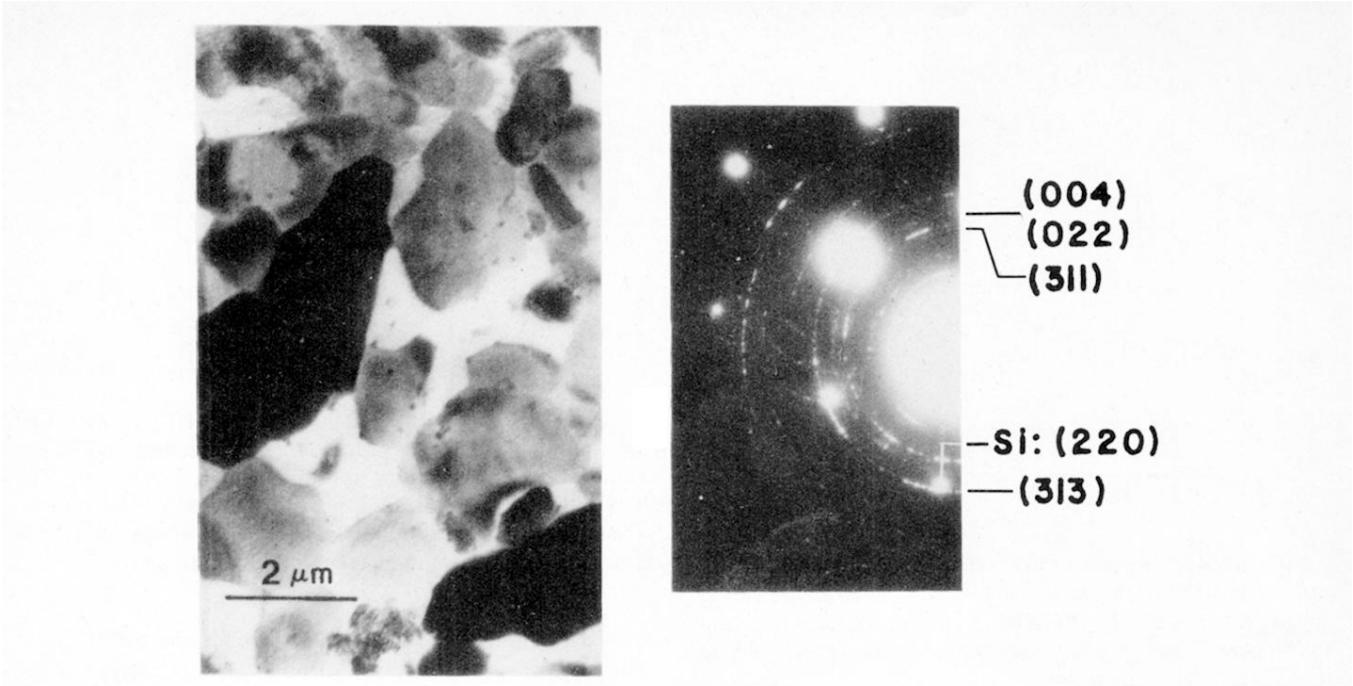
FIG. 8. (a) TEM bright field micrograph of a 200-Å Ti film on atomically clean Si(111) reacted at 650°C for 3 min; (b) corresponding diffraction pattern indexed for TiSi<sub>2</sub>.
