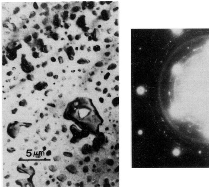
FIG. 11. (a) TEM bright field micrograph of a 100-Å Ti film on atomically clean Si(111) reacted at 300°C for 20 min and then at 780°C for 3.5 h; (b) corresponding diffraction pattern.
