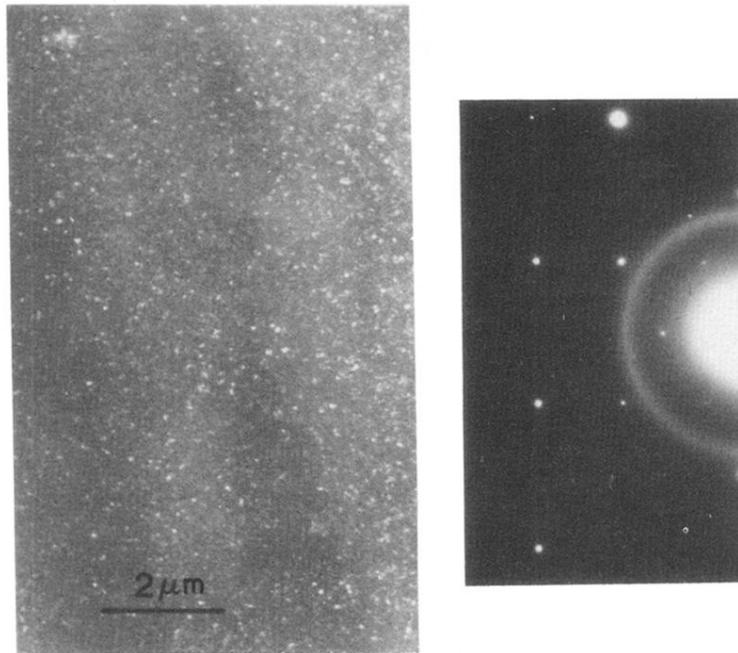
FIG. 10. (a) TEM dark field micrograph of a 100-Å Ti film on atomically clean Si(111) reacted at 300°C for 20 min; (b) corresponding diffraction pattern.
