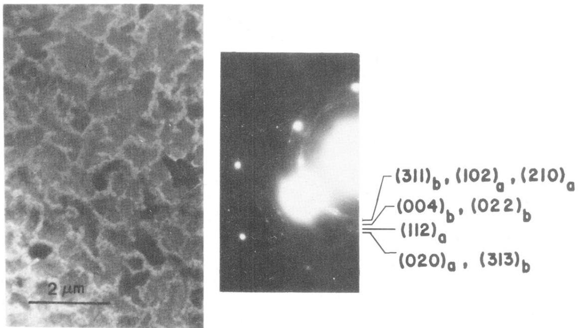
FIG. 9. (a) TEM bright field micrograph of a 30-Å Ti film on atomically clean Si(111) reacted at 600°C for 30 min; (b) corresponding diffraction pattern indexed for both TiSi (subscript *a*) and TiSi<sub>2</sub> (subscript *b*).
