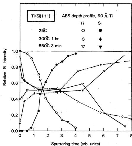
FIG. 6. AES sputter profiles of a 90-Å Ti film at 25°C, reacted at 300°C (1 h), and reacted at 650°C (3 min). The  $Ti\ L_{2,3}M_{2,3}M_{2,3}$  and  $Si\ L_{2,3}VV$  AES intensities are measured relative to pure Ti and pure Si, respectively, and the data are plotted in terms of relative Si intensity.
