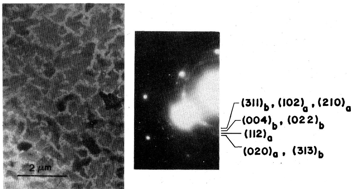
FIG. 9. (a) TEM bright field micrograph of a 30-Å Ti film on atomically clean Si(111) reacted at 600°C for 30 min; (b) corresponding diffraction pattern indexed for both  $\text{TiSi}$  (subscript *a*) and  $\text{TiSi}_2$  (subscript *b*).
