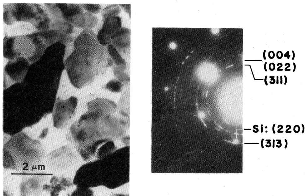
FIG. 8. (a) TEM bright field micrograph of a 200-Å Ti film on atomically clean Si(111) reacted at 650°C for 3 min; (b) corresponding diffraction pattern indexed for  $\text{TiSi}_2$ .
