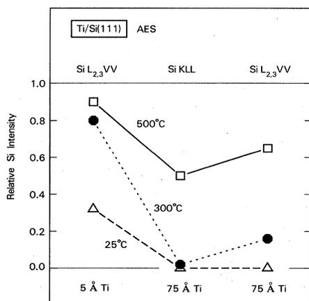
FIG. 4. AES intensity behavior of Si  $L_{2,3}VV$  and  $KLL$  for a fairly thick (75-Å) Ti film as a function of annealing temperature (10 min treatments) and as compared to a thin (5-Å) film.
