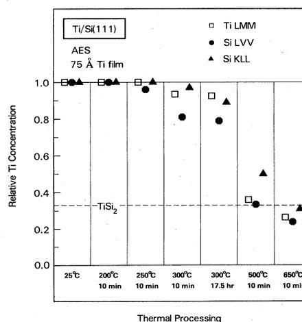
FIG. 5. AES intensity behavior of Si  $L_{2,3}VV$ , Si  $KLL$ , and Ti  $L_{2,3}M_{2,3}M_{2,3}$  transitions for a 75-Å Ti film as a function of annealing conditions. The Ti and Si AES intensities are measured relative to pure Ti and pure Si, respectively, and the data are plotted in terms of relative Ti concentration in the film (as opposed to Si concentration).
