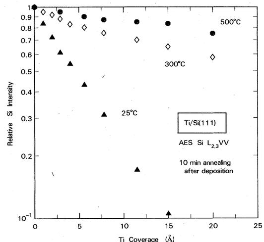
FIG. 1. AES intensity behavior of Si  $L_{2,3}VV$  as a function of Ti coverage at various temperatures. For the 300- and 500- $^\circ\text{C}$  cases, each data point corresponds to depositing more Ti at room temperature, annealing for 3 min at the elevated temperature, and remeasuring the intensity at room temperature.
