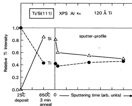
FIG. 7. XPS intensities [from  $Si(2p)$  and  $Ti(2p)$  core levels] for deposition of a 120-Å Ti film at 25°C, reaction at 650°C for 3 min, and sputter profiling with XPS into the overlayer. The XPS intensities are depicted relative to pure Ti and pure Si respectively, and the data are plotted in terms of relative Ti concentration in the film (as opposed to Si concentration).
