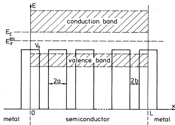
FIG. 1. One-dimensional metal-semiconductor-metal ( $M$ - $S$ - $M$ ) structure. The conduction and valence bands refer to an infinitely long semiconductor. Parameter values used in the calculations are  $V_0 = 7 \text{ eV}$ ,  $E_F = 7.75 \text{ eV}$ ,  $a = 2.26 \text{ \AA}$ , and  $b = 0.24 \text{ \AA}$ .
