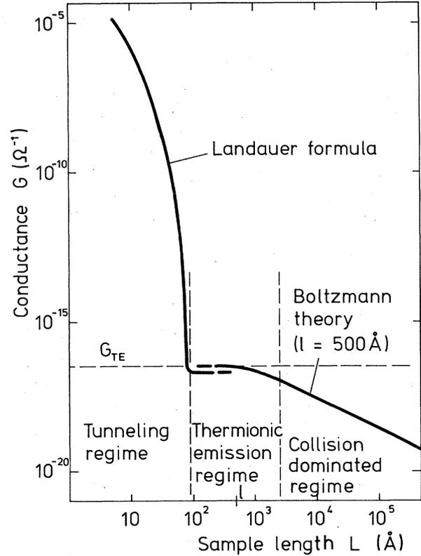
FIG. 2. Conductance of the one-dimensional metal-semiconductor-metal structure at  $T = 300 \text{ K}$  as a function of the length of the semiconducting region.
