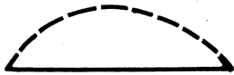
FIG. 1. Lowest-order diagram of the phonon scattering or of the exchange energy, where a dashed line represents the electron-phonon interaction or the electron-electron interaction, respectively; a full line represents the free-particle Green's function.
