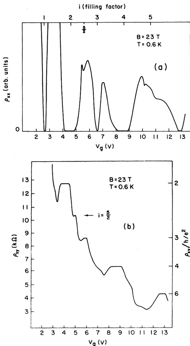
FIG. 4. Results at 23 T following change in density of interface states. (a) Longitudinal resistivity as a function of gate voltage. (b) Transverse resistivity as a function of gate voltage.
