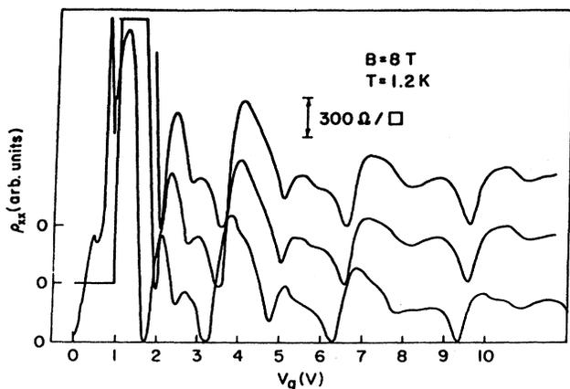
FIG. 1. Longitudinal resistivity as a function of gate voltage in the presence of slow interface states.
