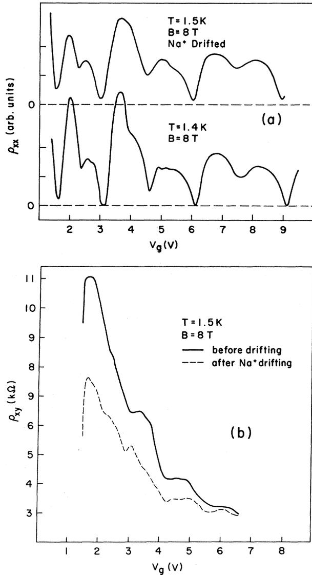
FIG. 2. (a) Longitudinal resistivity as a function of gate voltage before and after sodium drifting. (b) Transverse resistivity as a function of gate voltage before and after drifting.
