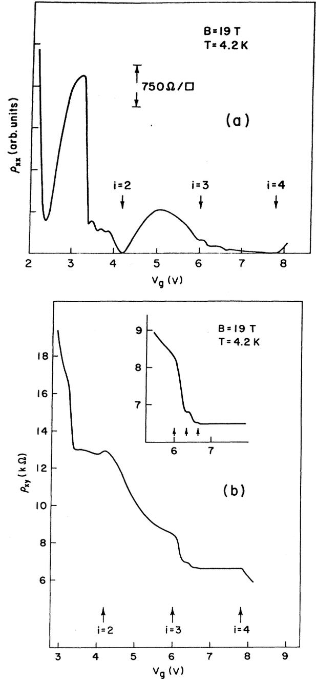
FIG. 3. Results at 19 T. (a) Longitudinal resistivity as a function of gate voltage. (b) Transverse resistivity as a function of gate voltage.
