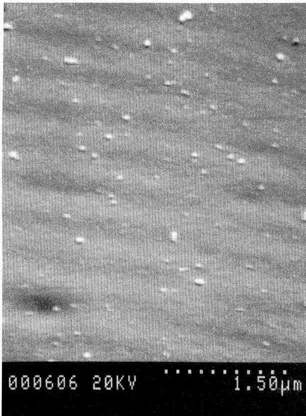
FIG. 12. Electron-microscope picture of the smoothly varying ripples formed by three s -polarized, 1.06\text{-}\mu\text{m} pulses incident at 45^\circ with fluences in regime D .
