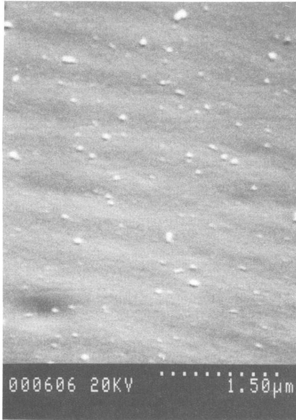
FIG. 12. Electron-microscope picture of the smoothly varying ripples formed by three s -polarized, 1.06\text{-}\mu\text{m} pulses incident at 45^\circ with fluences in regime D .
